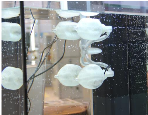
Fig. 17.7 FLM printed OSA with integrated hydraulic system.
