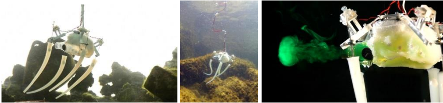
Fig. 21.3 Images of the PoseiDRONE prototype, from left to right: view of the 4-arm prototype in a salt water tank, the prototype in sea water, detail of the pulsed-jet propulsion with the fluorescein dyed vortex ring (credits to Massimo Brega, The Lighthouse).
