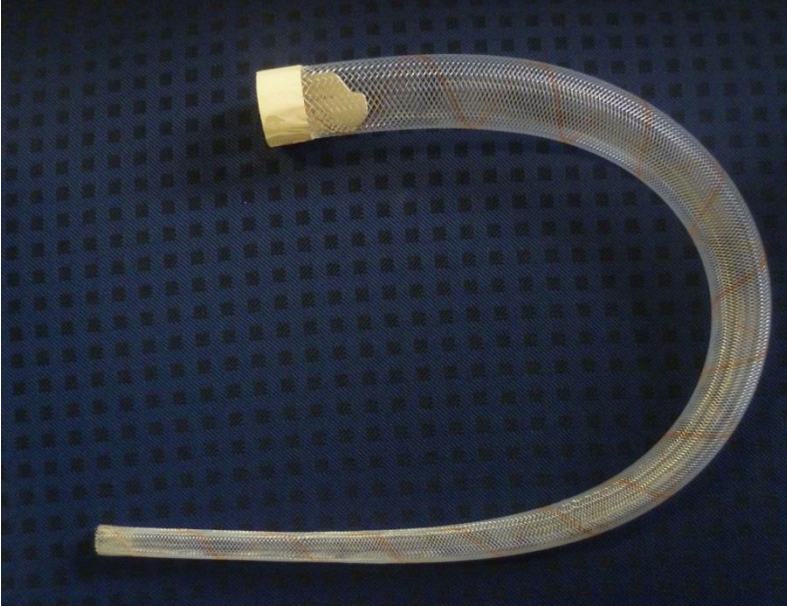
Fig. 14.3 Biaxial PET Monofilament braid used for the EU- project “Octopus”
