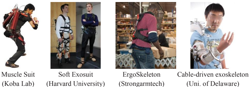
Fig. 5.6 Examples of state of the art wearable cable-driven robots
