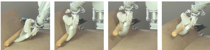
Fig. 18.10 Caging during of the slide-to-wall grasp strategy.
