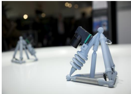
Fig. 17.4 Autonomous robot system with flexible and solid areas built in one single piece. The flexible zones is the bellow which is powered by a small air-pump.
