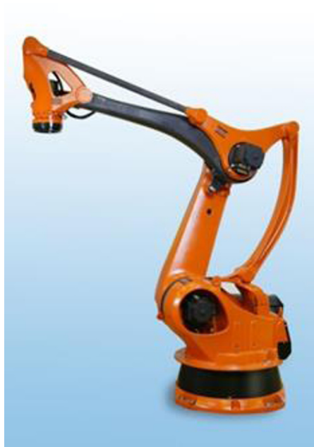
Fig. 14.8 Kuka - Robot with carbon composite arm
