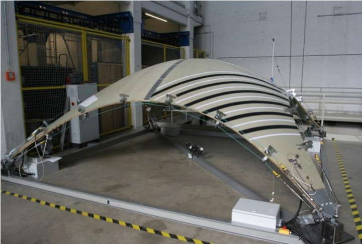
Fig. 14.19 Adaptive hybrid structure [C. Riethmüller, ITV/HIKE Stuttgart]
