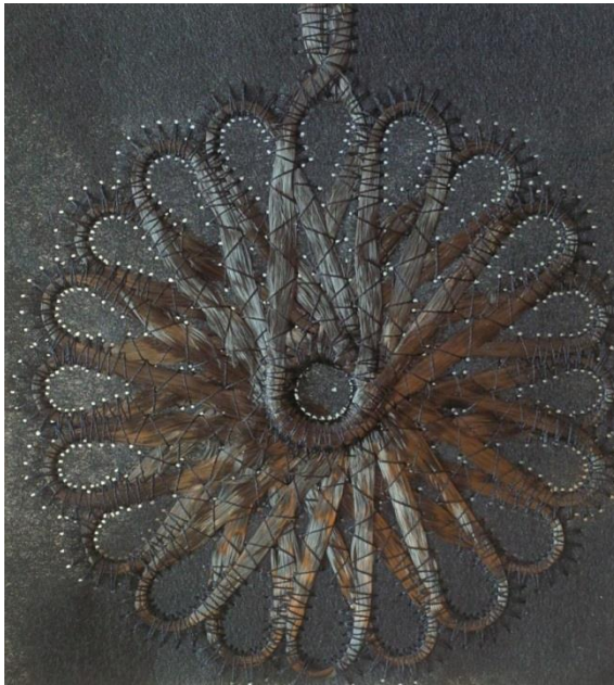
Fig. 14.1 Embroidery of Carbon Fibers to place the fibers along the load paths in the part. (Courtesy ACC Technologies, FS Software&Konstruktionen GmbH)
