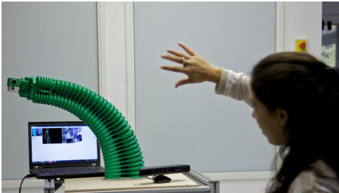
Fig. 17.5 Interactive CamBot with soft-actuator made of PA 12 (SLS).
