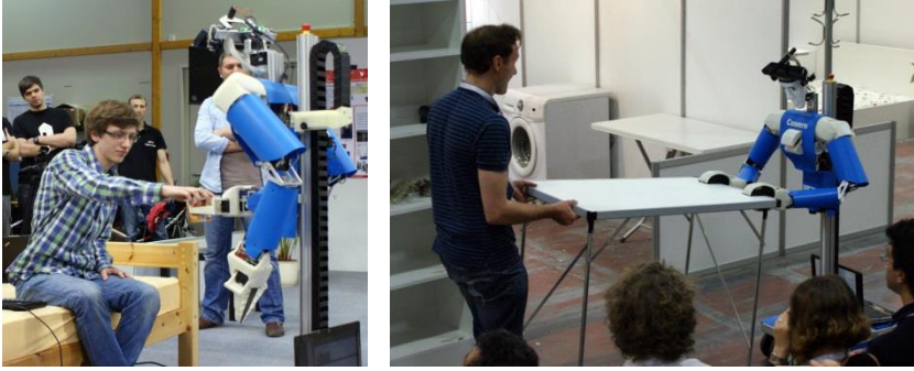
Fig. 7.2 Left: Cognitive service robot Cosero hands an object to a person. Right: cooperative carrying of a table by a person and Cosero.
