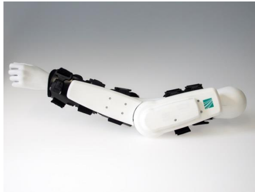
Fig. 16.3 Active Arm Orthosis CyberRehab by Fraunhofer IPA, Stuttgart, Germany
