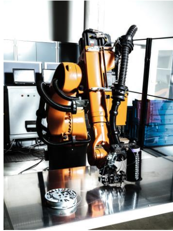
Fig. 17.9 FLM based robotic system: 3D Fibre Printer with build volume of 2m x 1m x 1m.
