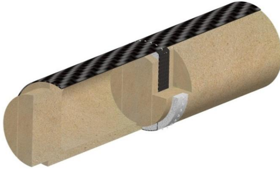
Fig. 14.14 Bamboo inspired nodal composite structure
