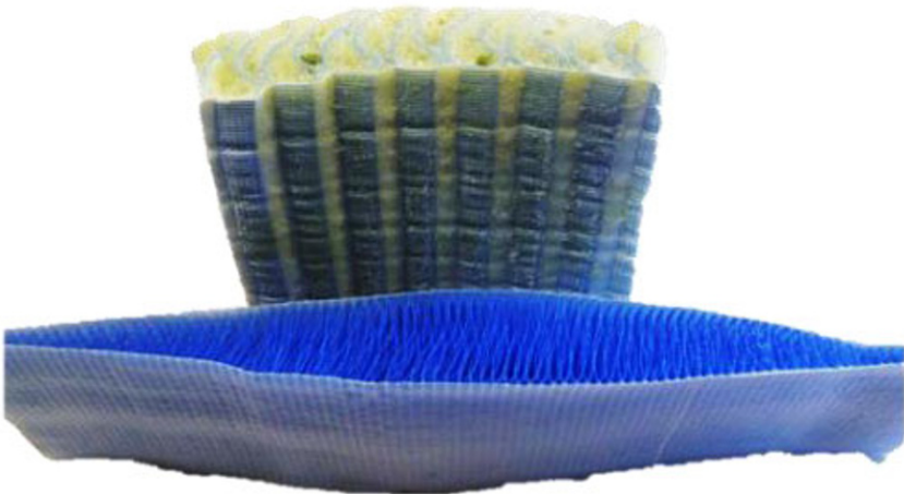
Fig. 14.7 3D woven lentil like structures inspired by sand dollar [H.J. Bauder, ITV]
