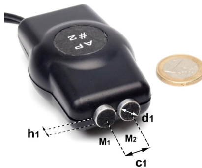
Fig. 1. Representation of the double headed acoustic probe. M_1 – Microphone 1; M_2 – Microphone 2; c_1 - distance between transducers centres: \approx 11 mm; d_1 : microphones diameter: 9.7 mm; h_1 : sensors external height: 2 mm.
