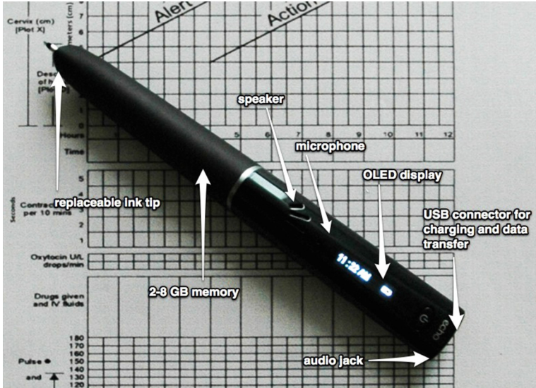
Fig. 2. The digital pen used in the PartoPen system is depicted. The speaker, microphone, OLED display, USB connector, audio jack, memory storage, and replaceable ink tip are identified.
