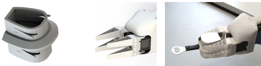
Fig. 3. Tool Adapters. We designed special adapters for tools to establish stable grasps that resist forces and torques in any direction. Left: Adapter attached to bottle opener. Center: Cosero’s gripper design. Right: Grasp on the bottle opener adapter.
