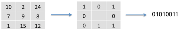
Fig. 4. Example of computing LBP_{8,1} pixel neighbourhood (left); threshold version (middle); resulting binary code (right).
