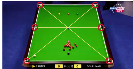
Fig. 4. Finding the position of middle pockets as lying on the intersection of diagonals
