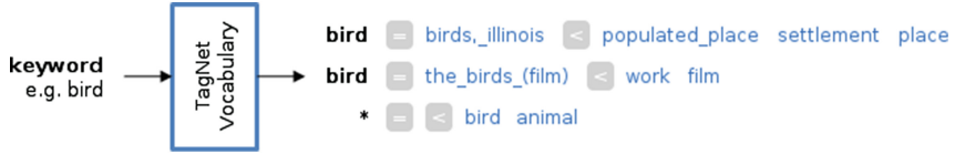
Fig. 2. A vocabulary takes a keyword as input and outputs one or more sematags.
