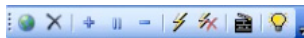
Fig. 2. ACTIVESHEETS Controls. Buttons from left to right: connect to and disconnect from the server, add a stream (‘+’ icon), pause a stream (pause symbol), disconnect from a stream (‘-’ icon), export data back to the server (flash symbol), stop data export (crossed out flash symbol), export computation (movie symbol), and lastly, debug mode (light bulb), used to debug the implementation of ACTIVESHEETS .
