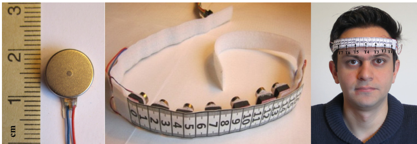
Fig. 2. Left: Pancake type vibration motor, Center: Tactile headband interface, Right: A participant wearing the tactile headband interface.
