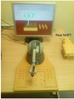
Fig. 1. The rig set up used in our study shows the wooden housing rig, the Phantom Omni, the real rig and a sample of a screen shot on the VDU.
