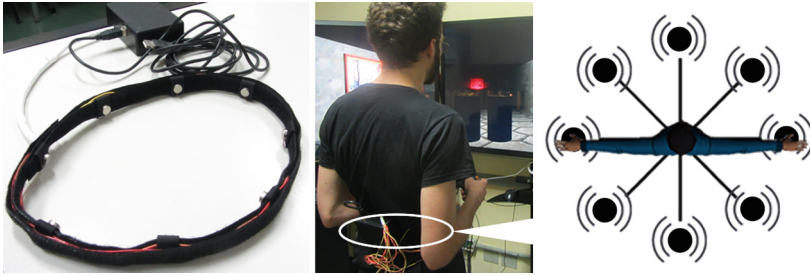
Fig. 1. The vibrotactile belt. In the middle, a participant using the belt to navigate. In the right, a top view of a humanoid showing the vibrators positioned at equidistant locations around the waist.
