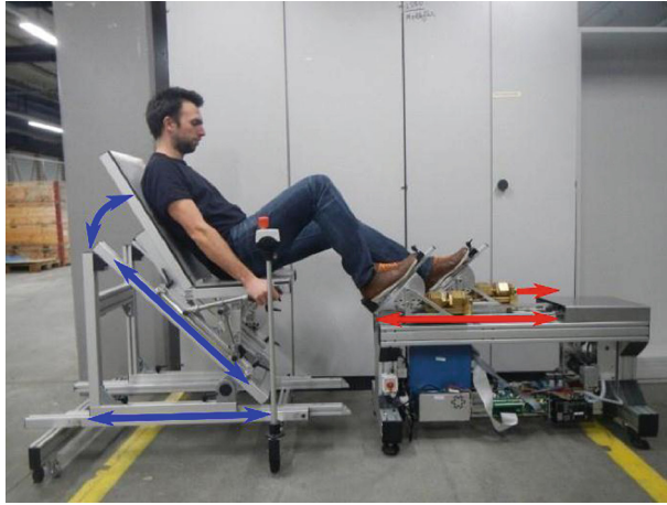
Fig. 1. The LegoPress. The red arrows represent the actuated degrees of freedom while the blue ones are the possible pre-defined settings on the chair (Color figure online).
