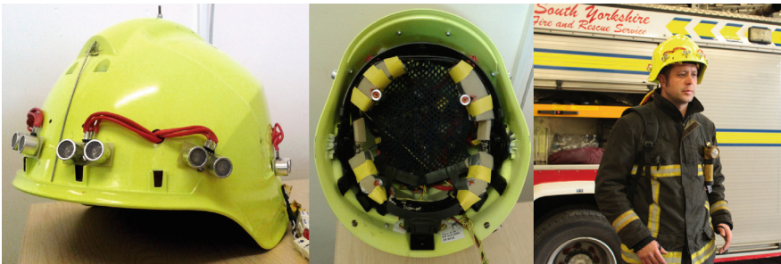
Fig. 1. The tactile helmet: a prototype sensory augmentation device developed to assist fire-fighters navigating in smoke-filled buildings [4].
