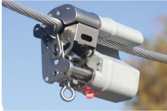
Fig. 3 Sentient Energy's Advanced Monitoring Platform (All rights reserved)
