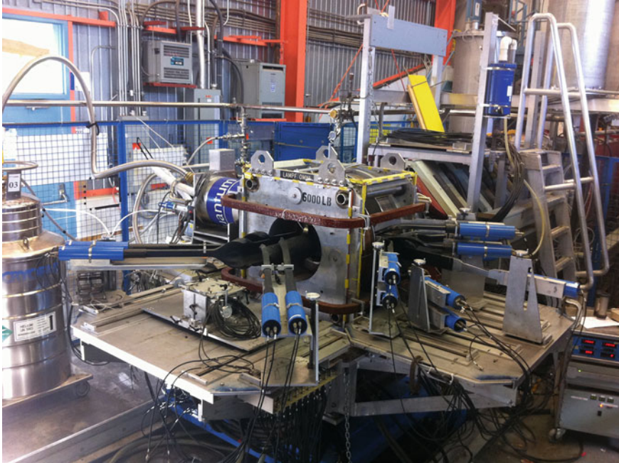
Fig. 8.2 A photograph of a \mu SR spectrometer at TRIUMF. A large Helmholtz coils are used to generate magnetic field parallel to the muon beam direction, while sets of smaller coils are used to generate magnetic field perpendicular to the muon beam direction. The specimen is placed in the center of these coils within a Helium gas flow cryostat which has horizontal access (shown by the silver/blue cylindrical object ). Blue tubes contain photo-multipliers connected to black light guides and plastic scintillation counters for detecting muons and positrons. In the top-right corner of the picture is shown a part of high-voltage generator of a spin rotator (Wien filter) with which the spin polarization direction of incident muons are rotated from the original direction parallel to the muon flight direction. One sees a part of beamline quadrupole magnets guiding the muon beam to the location of the specimen. This picture was taken at the M15 beamline of TRIUMF. Other instruments for \mu SR measurements can be seen at web pages of TRIUMF [110], PSI [111] and ISIS [112] muon facilities
