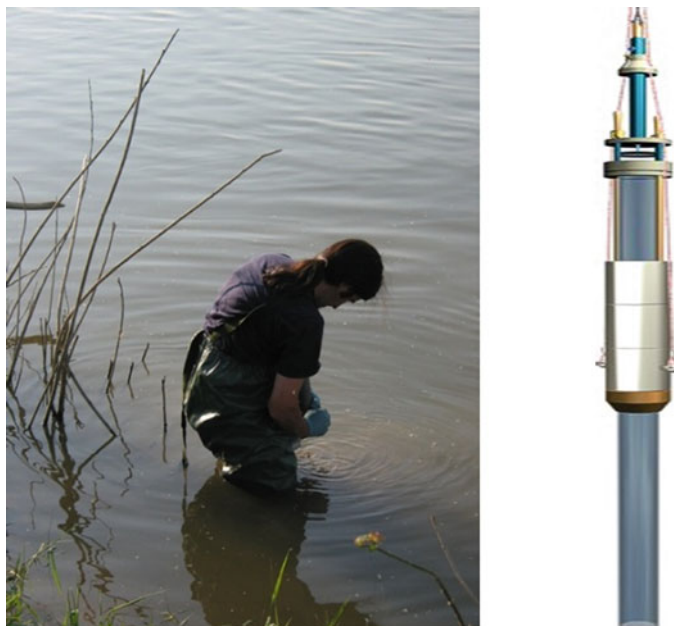
Fig. 2 Sediment sampling and piston corer used for sampling of sediments
