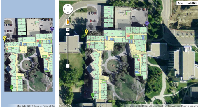
Fig. 2. Google Maps floor plan program example to add floor plan to traditional outdoor Google Maps
