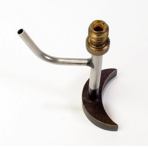
Fig. 4.12 Custom-made half moon probe for vascular lesion under the tongue
