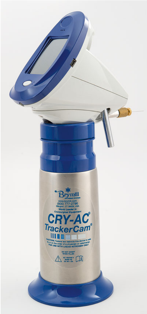
Fig. 4.8 The Cry-Ac ® TrackerCam (Brymill) which measures skin temperature and records the settings and procedure (Courtesy of Brymill Cryogenic Systems)
