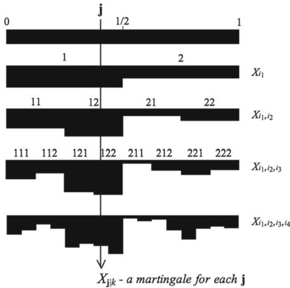
Fig. 7 A random multiplicative binary cascade measure represented on the interval [0, 1] , with X_{j|k} a martingale for each j \in [0, 1]
