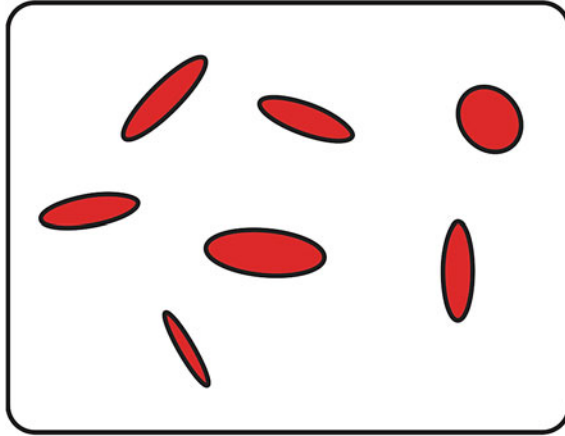
Fig. 7.4 RVE with ellipsoidal inclusions
