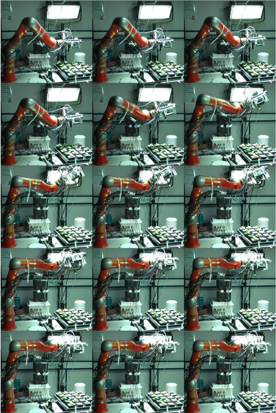
Fig. 8.6 Explorative learning of inverse kinematics for reaching on a 7 DoF robotic arm
