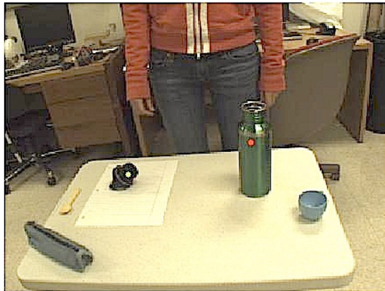
Fig. 5.4 Example result of object detection with SVM classifier using HoG features. Dots indicate detected object centers.
