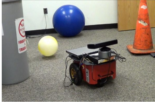
Fig. 2.9 Our robot tracking a ball in real-time only using only 3D range data from MS Kinect (307200 points)
