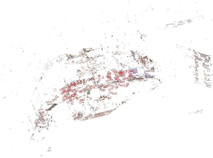
Fig. 7.2 Estimated camera poses and sparse 3D reconstruction in the Indoor dataset that is used for evaluating LBA and BA probability distributions
