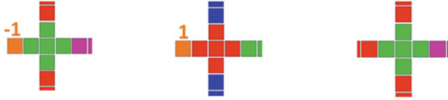
Fig. 6. QCA majority gates, with and without one fixed input, and associated clocking. The majority gates with cell polarizations fixed as -1 and +1 function as two-input AND or OR gates, respectively.
