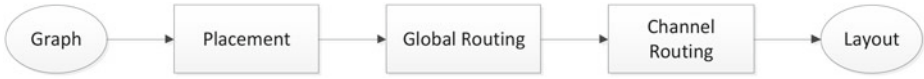
Fig. 13. Physical Mapping flow diagram. The circuit layout is generated starting from its graph following several optimization steps.
