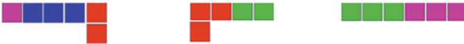
Fig. 4. Three example sections of QCA wires with “90-degree” cell orientation, two of which include right angle corners.
