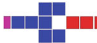
Fig. 5. A complex inverter with two-cell input and output legs and specified clock zones.
