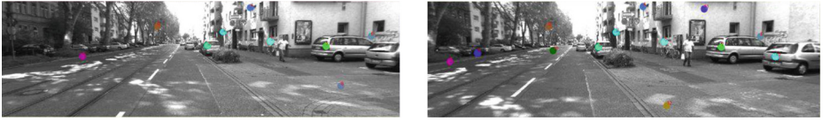
Fig. 3. (Left) At frame 60 features are initialized. (Right) At frame 70, features tracking result.
