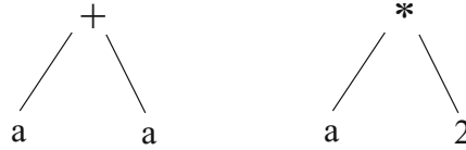
Fig. 7.4. Example of two equivalent solution trees, generated by different terminal and function sets. The left-hand side tree is generated from F = \{+\} , T = \{a\} , and the right-hand side tree is generated from F = \{*\} , T = \{a, 2\}
