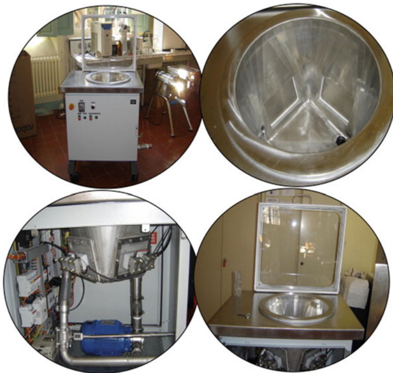
Fig. 13.6 Pilot plant-scale model of 30 L volume UAWE apparatus: general view, inside of the reactor tank, recirculating pump and outside bottom of the reactor, top of the reactor with opened protection door (Reprint from [11] with permission from Elsevier)
