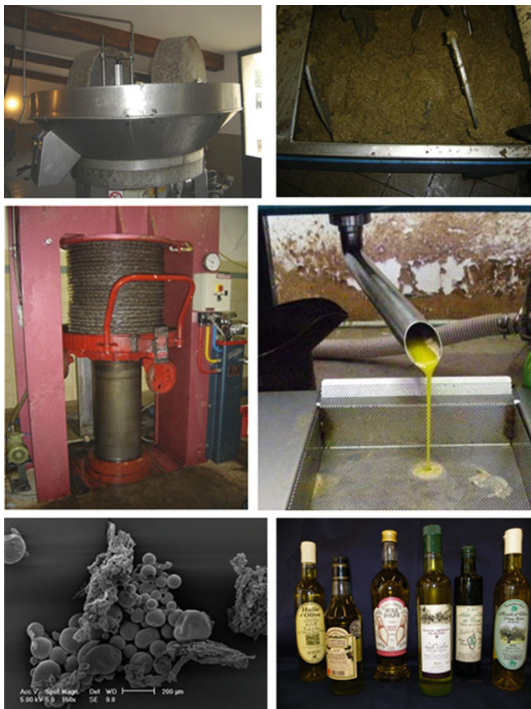
Fig. 2.1 Solvent free olive oil extraction process
