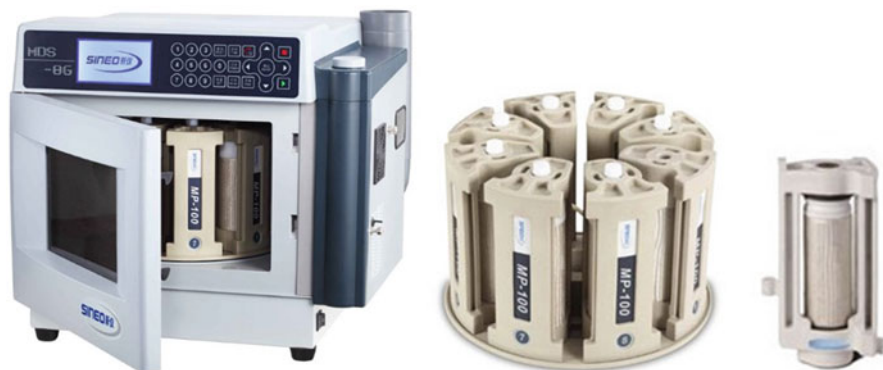
Fig. 13.8 Closed-vessel microwave chemistry workstation (MDS-8G model, Sineo Co., China)
