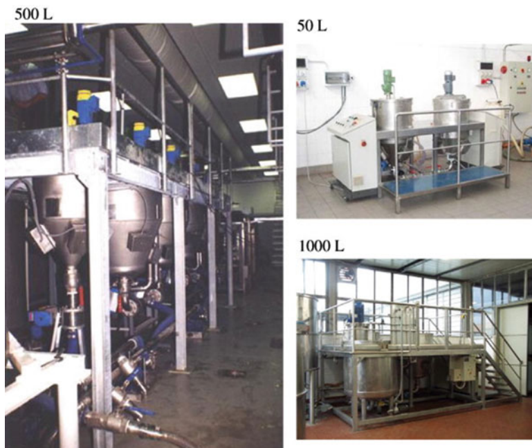
Fig. 13.3 Industrial-sale UAWE equipments with 50, 500, and 1,000 L reactor tank capacities (Reprint from [1] with permission from Elsevier)
