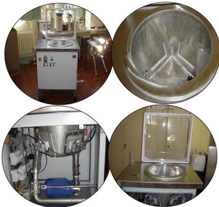
Fig. 13.6 Pilot plant-scale model of 30 L volume UAWA apparatus: general view, inside of the reactor tank, recirculating pump and outside bottom of the reactor, top of the reactor with opened protection door (Reprint from [11] with permission from Elsevier)
