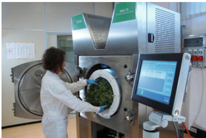
Fig. 13.11 Semi-industrial-scale MAE apparatus MAC-75 model (Milestone Inc., reprint from [28] with permission from Elsevier)
