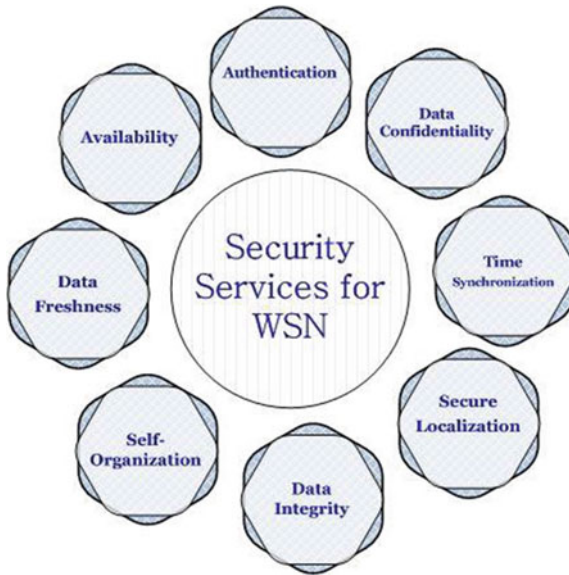
Fig. 11.1 Security services required for wireless sensor networks
