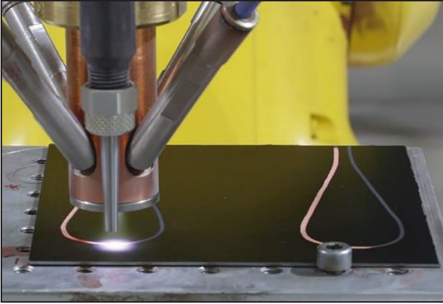
Fig. 8. Metal substrate coated with a cathodic dip paint (black) mounted on a robot-controlled sample stage. Selective metallization is accomplished by; 1) meticulously sandblasting and roughening the paint (thin nozzle in front), and 2) depositing copper and constantan via plasma deposition. Note the adhesion promoting structures (grey lines) with a width of approx. 1 mm and the as-deposited copper thermo legs (brown). Lateral track accuracy is within 0.2 mm.
