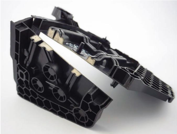
Fig. 10. Topology-optimized semi-structural lightweight part using a 2-C sandwich injection moulding process
