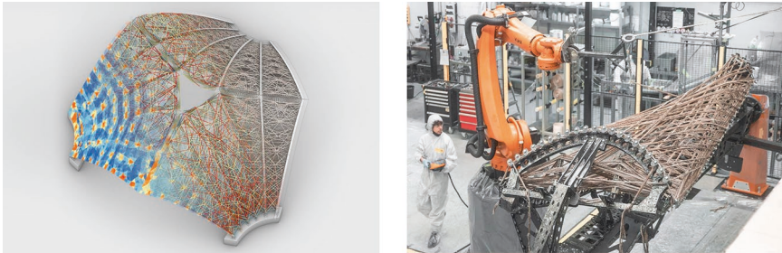
Fig. 6. Resource-efficient lightweight constructions through digital planning and manufacturing by means of winding (core-less winding) “More form – less material”. ©ICD/ITKE/IntCDC University of Stuttgart
