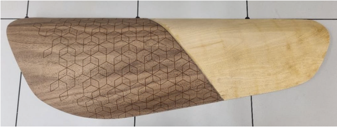
Fig. 2. A veneer based door panel with laser structured walnut top layer before applying the vegan leather.
