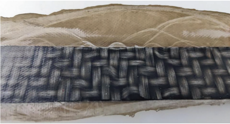
Fig. 6. Undulation and leaked matrix in refurbished specimen
