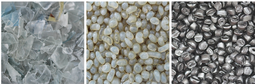
Fig. 7. Left: rPET flakes as supplied, Center: After re-granulation without additives, Right: Processed with additives
