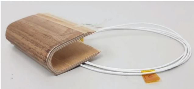
Fig. 3. Veneer sample with an integrated sensor.
