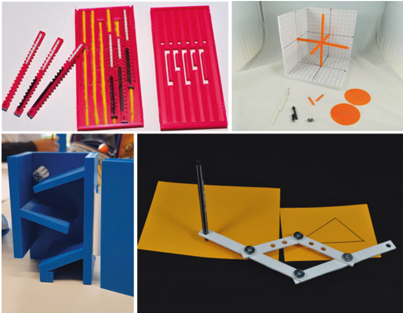
Fig. 7 Examples of 3D printed manipulatives (Clockwise from top left: A mechanical addiator or add/subtract calculator, a vector representation model, a pantograph, and a dice tower)
