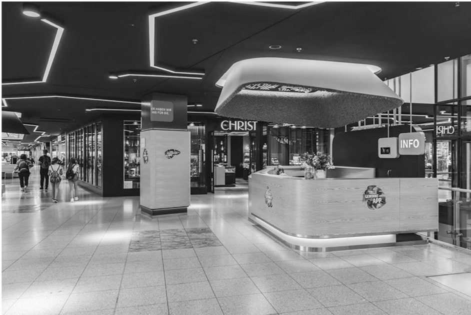
Fig. 21.4 Direct lighting above central places such as the customer information desk. (Courtesy of © LAGO Shopping-Center Konstanz 2020. All Rights Reserved)
