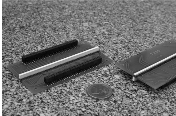
Fig. 14.2 Photodiode rows on both sides of a circuit board, each covered with scintillator of different thickness (Factory photo: PerkinElmer Optoelectronics)
