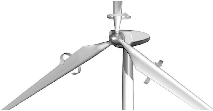
Fig. 3.101 Control of the pitch angle of the rotor blades of a wind turbine
