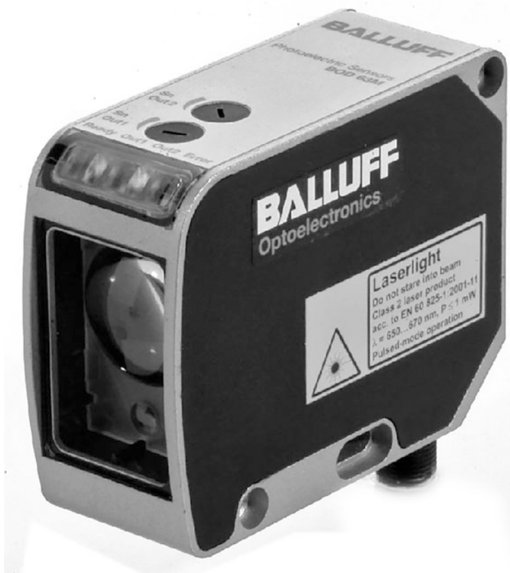
Fig. 3.54 Optoelectronic distance sensor of laser class 2 according to the pulse transit time method (front dimensions 35 \times 70 mm, factory photo: Balluff GmbH)
