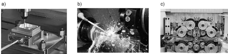
Fig. 4.10 Force sensors in the production process (a) measurement of the cutting force, (b) tool monitoring, (c) control of the roll forces (Factory photos: Kistler)
