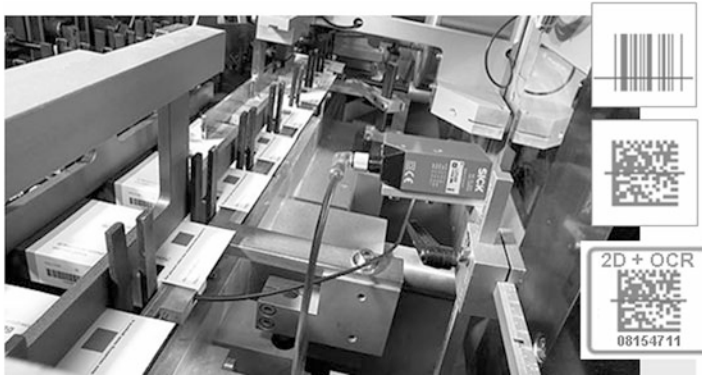
Fig. 3.201 Packaging industry: Counterfeit detection of goods and especially drugs code reading and character recognition: Serial number and date code
