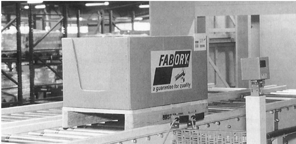
Fig. 3.186 Fixed-mounted bar code scanner for identifying moving objects (Factory photo: Sick AG)
