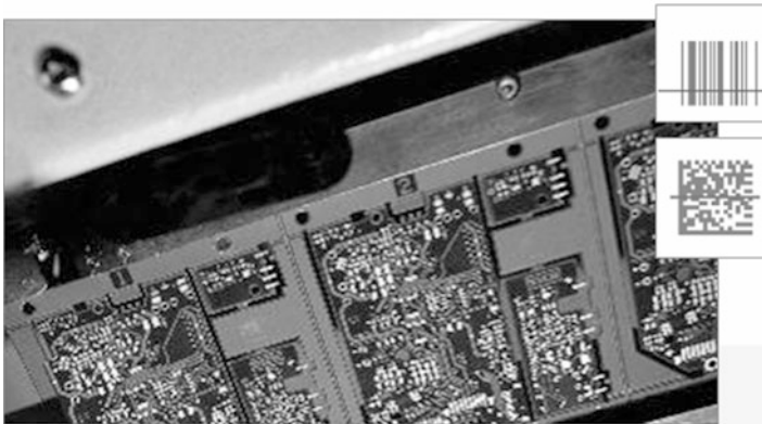
Fig. 3.200 Electronics manufacturing: Traceability of components, used in module production for tracking and identifying electronic cards and components
