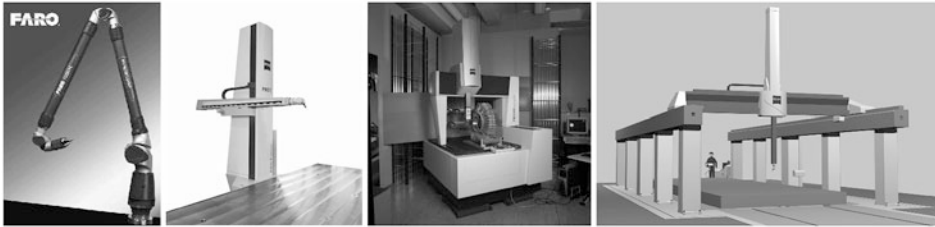
Fig. 3.212 Common coordinate measuring machines with different requirements and accuracies. From left to right: Articulated arm, horizontal arm coordinate measuring machine, gantry coordinate measuring machine, gantry coordinate measuring machine (Factory photos: Faro Technologies Inc., Carl Zeiss IMT GmbH)
