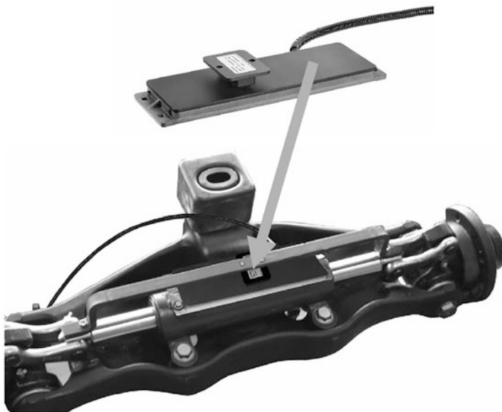
Fig. 3.34 Sensor mounted on steering cylinder; position sensor mounted on movable bracket (Factory photo: Novotechnik)
