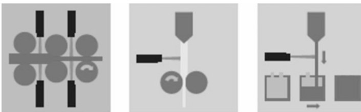
Fig. 6.18 Applications of stationary pyrometers in manufacturing (Source: Optris)
