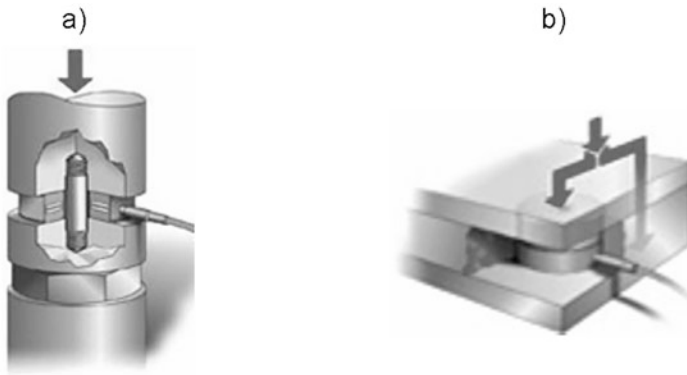
Fig. 4.4 Arrangements for force measurement (a) Direct force measurement; (b) Indirect force measurement (Factory photos: Kistler)
