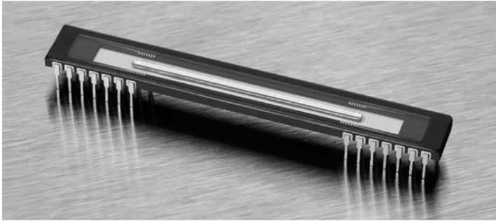
Fig. 14.15 CCD line sensor for use in spectroscopy (Factory photograph: PerkinElmer Optoelectronics)
