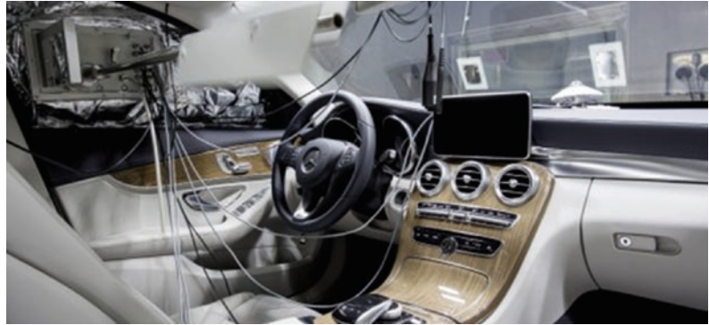
■ Fig. 8.37 Vehicle equipped with gas sensors to objectify the emissions of the components used. (Source: Daimler Global Media Site)
