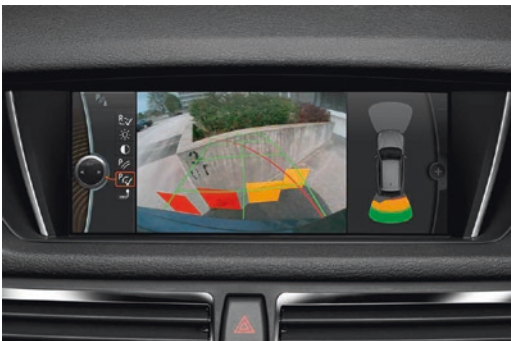
■ Fig. 9.12 Actual and target driving hose display superimposed on the rear view camera for parking (example: BMW)
