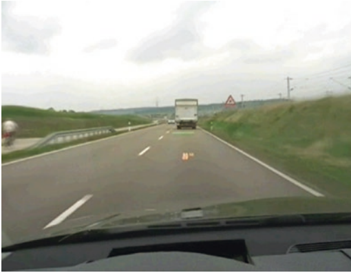
■ Fig. 9.28 Contact analog HUD (kHUD) with spacer bar (prototype Audi)
