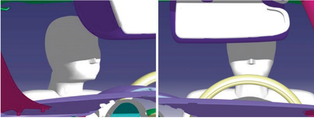
■ Fig. 7.77 Principle effect of the sun visor
