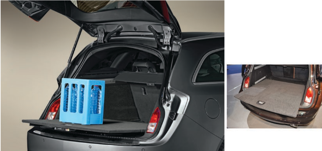
■ Fig. 7.118 Extendable loading floor of the Opel Insignia Sports Tourer (2013)
