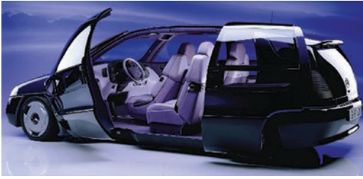
■ Fig. 7.96 Mercedes-Benz F100 research vehicle with centrally positioned driver's seat and sill that enters the car floor to facilitate access to the vehicle
