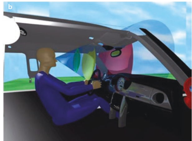
■ Fig. 7.55 Minimum viewing distances in the vehicle: a age-related loss of accommodation, b Distances in the vehicle for 50-year-old mid-size driver. (From Remlinger 2013)
