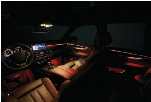
■ Fig. 8.8 Ambient lighting in door leaf. For ambient lighting, blue light should be avoided, as light adaptation is mainly done by the blue light sensitive cones. (Source Hella)
