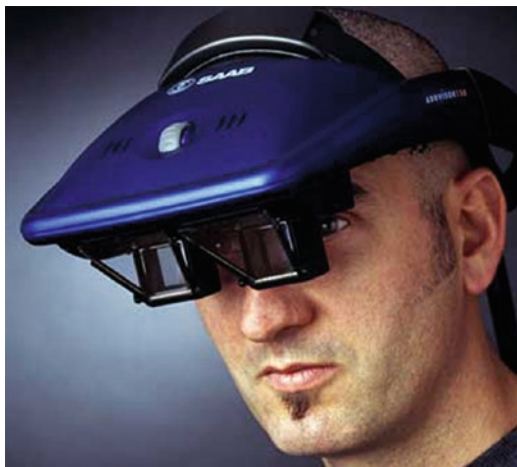
Fig. 10.17 Optical See Through HMD Saab AddVisor (SAABTECH 2006, from Bock 2008)
