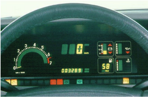
■ Fig. 6.10 Example of a digital speed display and mileage of the vehicle in 7-segment design
