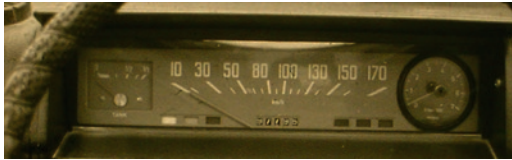
■ Fig. 6.12 Poor interpolatable nonlinear scale division. The example also shows that the center of the circular scale must coincide with the pointer pivot point
