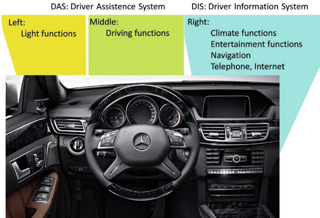
■ Fig. 1.8 The division of the dashboard area into DAS (Driver Assistance System) and DIS (Driver Information System), which came to a quasi-convention today
