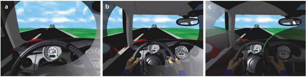
Fig. 7.52 Maximum driver field of view: a View of a small woman (FSMM), b View of a medium-sized man (MMMM), c Vision of a medium-sized man with varifocals. (From Remlinger 2013)
