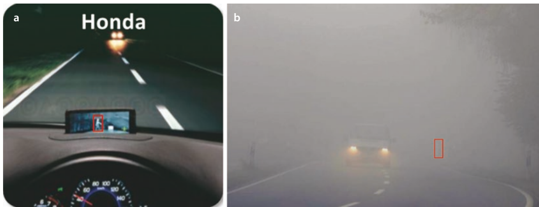
■ Fig. 6.17 Contact analog display to identify a pedestrian by means of an infrared night vision device, a on the display of a screen (example Honda), b directly in the real view according to a proposal by Bergmeier (2009)
