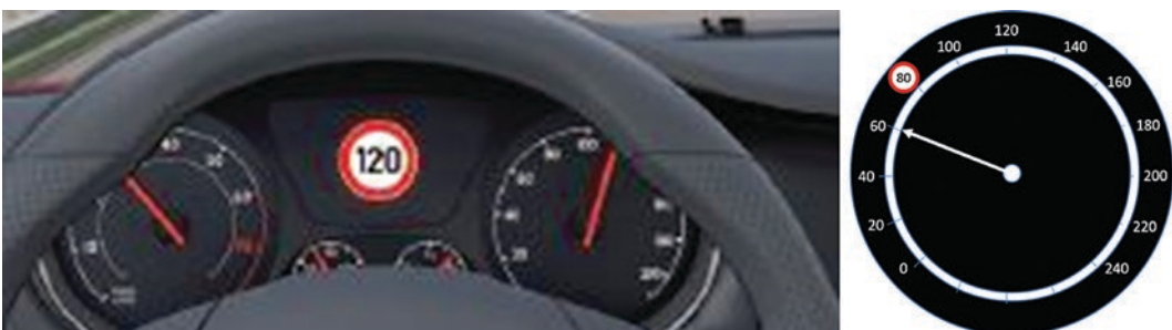
■ Fig. 9.1 Display of the speed limit by the traffic sign recogniser a Example Bosch, b Ergonomics proposal
