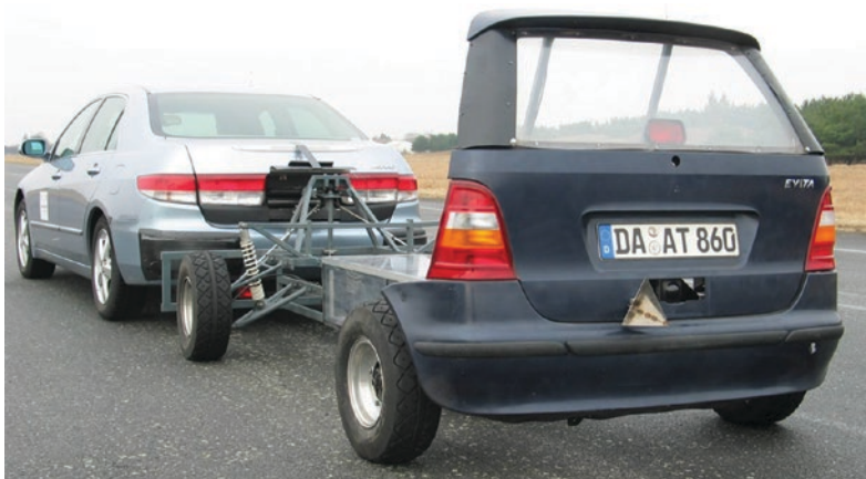
■ Fig. 10.21 Target vehicle with EVITA trailer, which prevents collision with the test vehicle even under extreme conditions. (Source: Fahrzeugtechnik, TU-Darmstadt)
