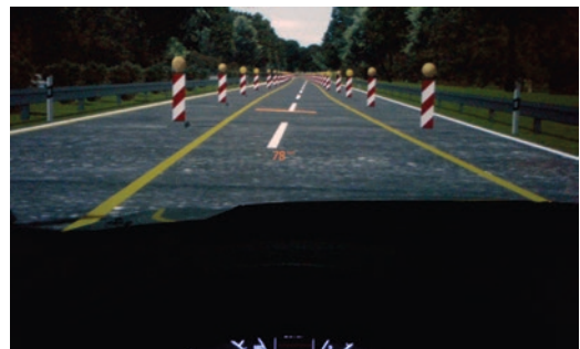
■ Fig. 6.42 Display of the driving hose in the contact-analog HUD; the lateral position of the reflected bar indicates where the vehicle is in 1.5 seconds, if no corrosive control element interventions are made
