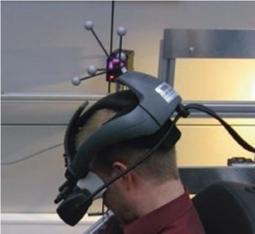
■ Fig. 11.4 Marker arrangement for detecting the spatial orientation of a body element
