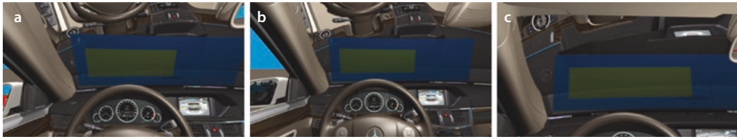
■ Fig. 7.75 Calculations of the reflection of the dashboard surface in the windshield for the little woman (a FSMM), the medium-sized, long-legged man (b MMML) and the tall man (c MTMM). The viewing cone is directed towards the so-called A-field (dark
