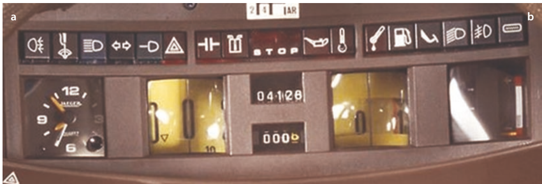
Fig. 6.15 Magnifying glass tachometer a and rev counter b in the Citroën CX
