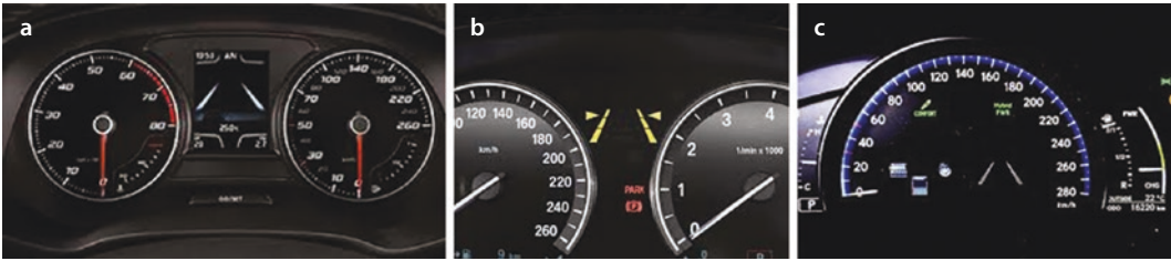
■ Fig. 9.6 Feedback via the activated LDW or LK S system (a Volkswagen, b BMW, c Mercedes)
