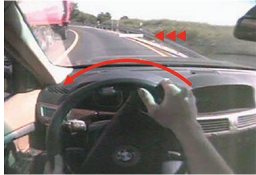
■ Fig. 9.29 Display of a necessary lateral guide correction in the cHUD (Lange 2008)
