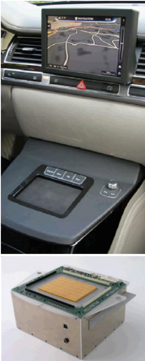
■ Fig. 6.35 Concept of the haptic touchpad (Spies et al. 2010; Spies 2013)
