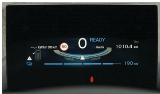
■ Fig. 6.37 Display of speed, current energy consumption and range (example: BMW i3)
