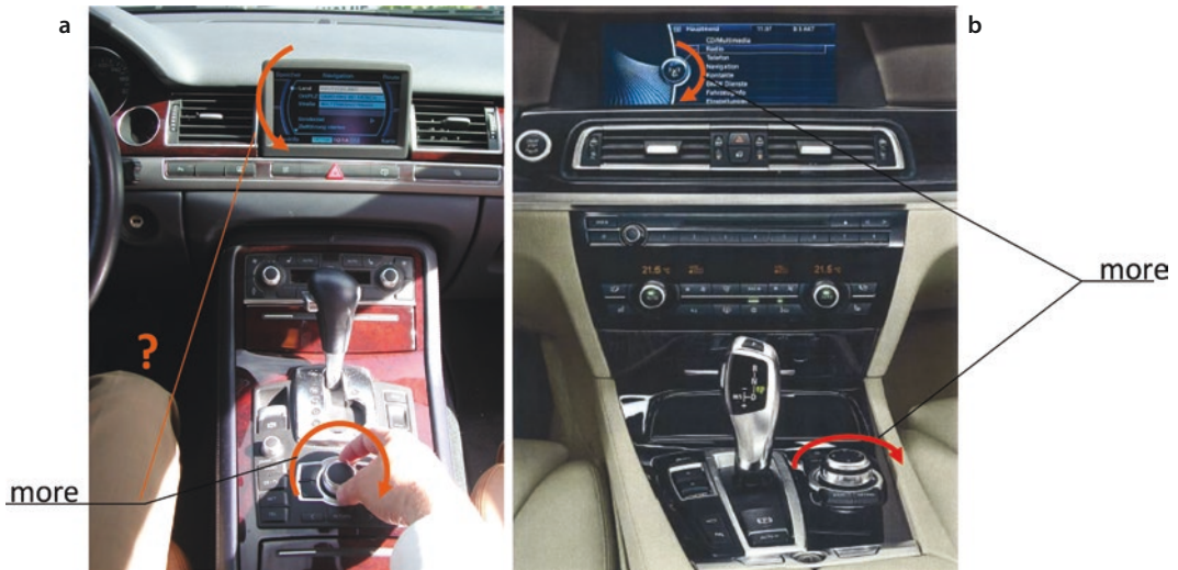
Fig. 6.29 Incompatibility a between the rotation of the controller and the reaction on the screen and the solution of the conflict b
