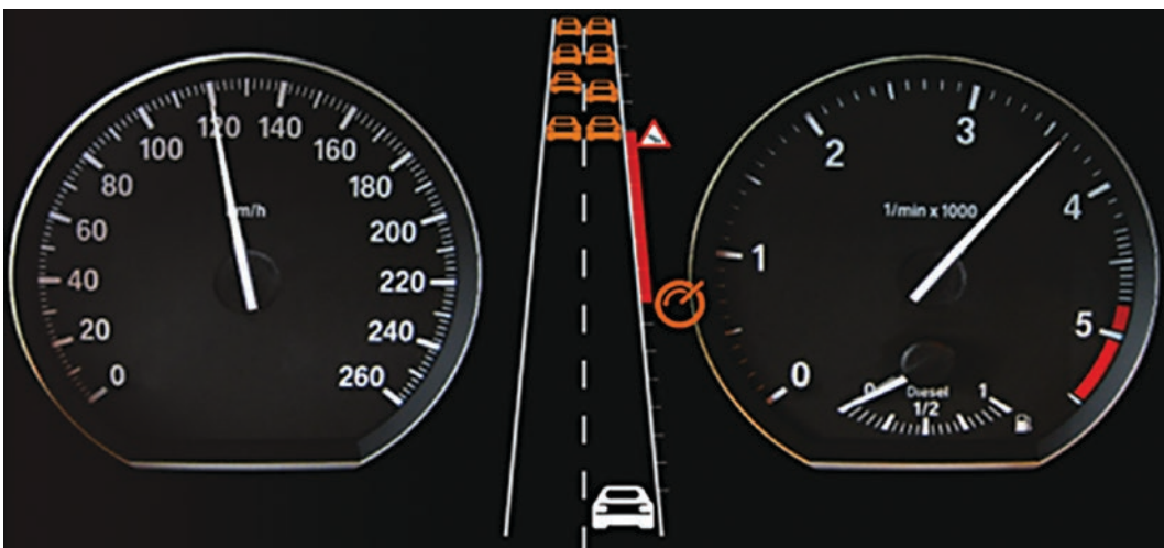
■ Fig. 9.16 Bird-view indicator for approaching the end of a traffic jam (Popiv 2011)
