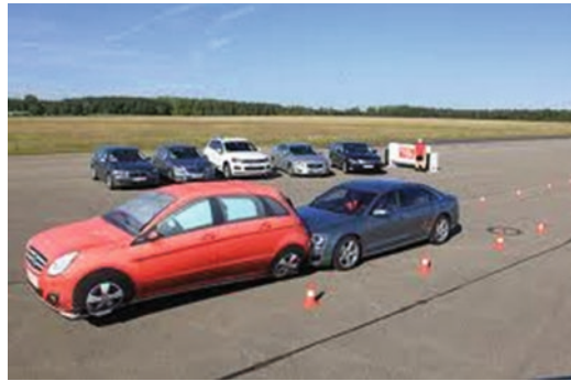
■ Fig. 10.20 Using an air car to check the effectiveness of the emergency brake assistant
