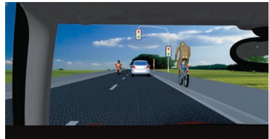
■ Fig. 7.56 Parametrically adjustable traffic situation with road users and objects for visual analysis in connection with a given 3-D CAD geometry. (From Remlinger 2013)
