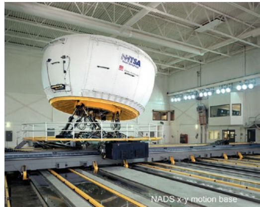
■ Fig. 10.14 NADS simulator on hexapod and x-y traversing carriage for the simulation of kinesthetic stimuli using wash-out effects
