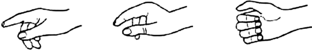
■ Fig. 6.30 Types of grip (according to Götz 2007); contact (index finger), grasping (two or three fingers) and grasping grip
