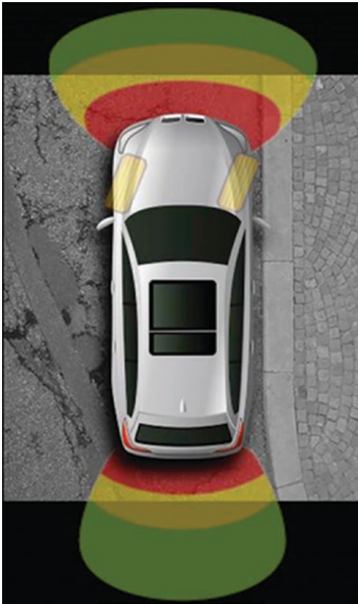
■ Fig. 9.11 All-round camera image combined with parking distance display (PDC) (Doisl 2008)
