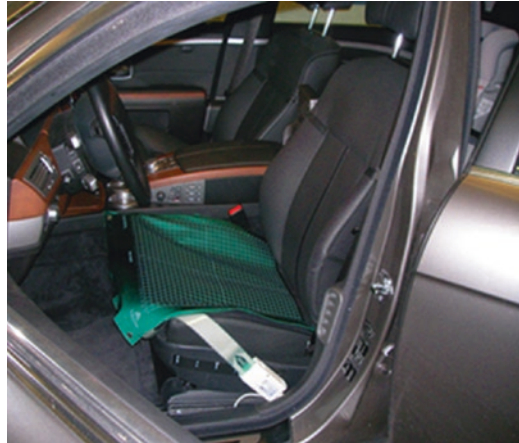
Fig. 11.7 Seat pressure mat in a vehicle seat
