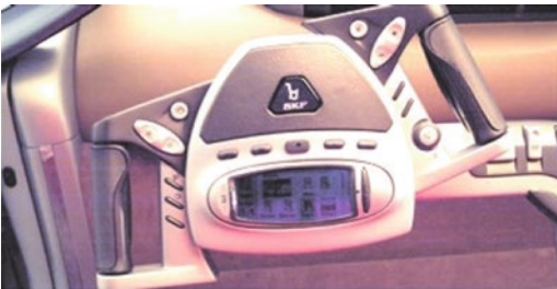
■ Fig. 6.67 Filo control element for longitudinal and lateral guidance of Bertone and SKF (2001)
