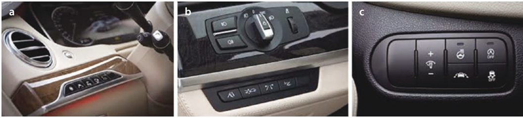
■ Fig. 9.5 Examples of assistance system control units (a Mercedes S-Class, b BMW 7 Series, c Volkswagen Golf)
