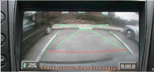
■ Fig. 6.18 Reversing assistance with faded-in auxiliary lanes for parking, which takes into account the above recommendations
