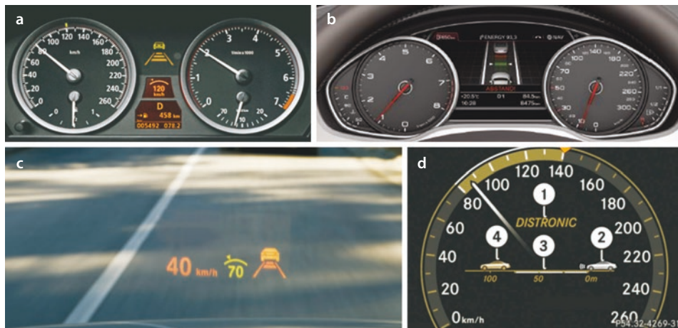
Fig. 9.3 Feedback on the operating status of the ACC (BMW E60, a or Audi b and Mercedes Distronic plus d using a pictorial display. In the optional HUD
