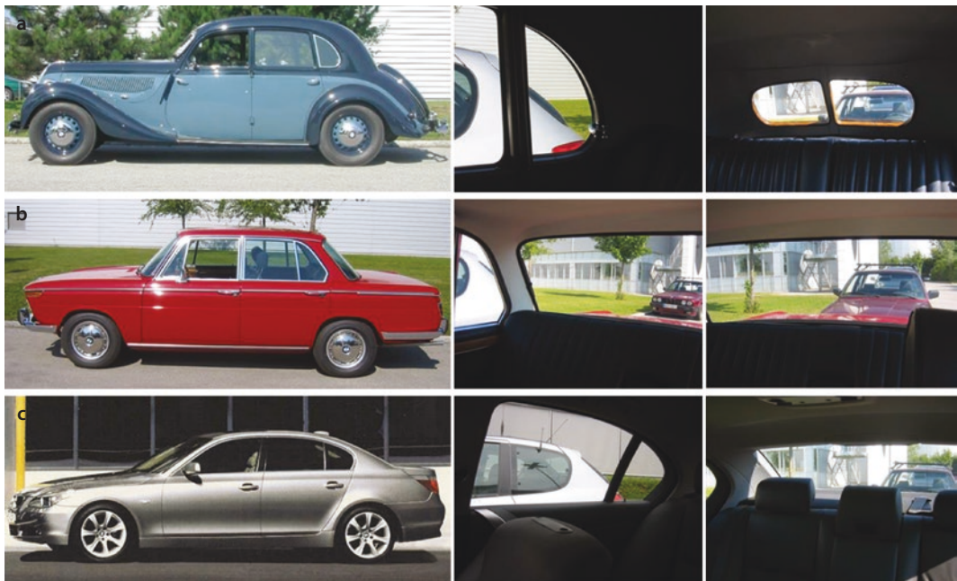
Fig. 7.61 View diagonally backwards (centre) and backwards (right) for three vehicles of different design generations. a BMW 326 year of construction 1938, b BMW 2000 year of construction 1968, c BMW 520i Year of construction 2002
