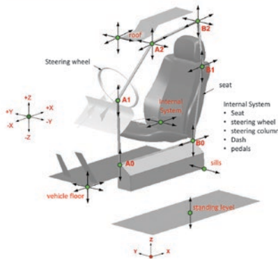
■ Fig. 7.110 Variable entry model (VEMO) for systematic research of entry behaviour. (Built at BMW, from Cherednichenko 2007)
