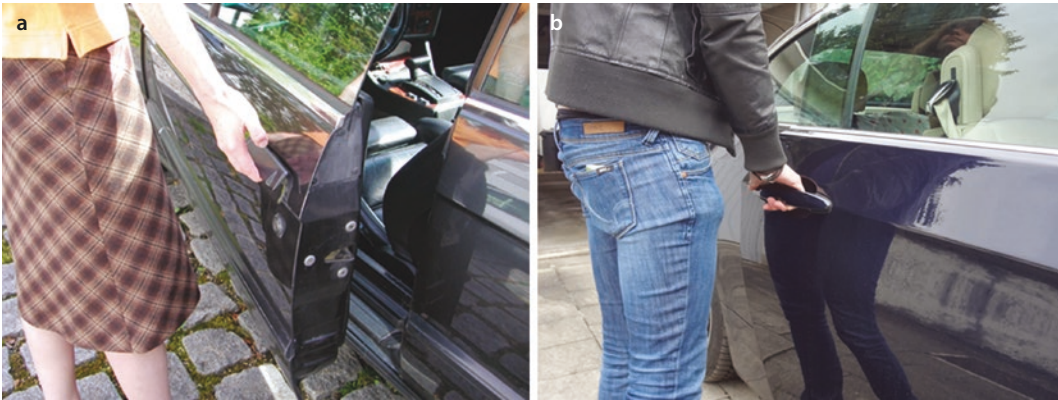
■ Fig. 7.97 Door handle as lifting plate (a) or as a handle (b)
