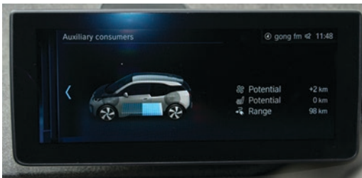
■ Fig. 6.40 Display of additional range potential by switching off consumers (example BMW i3)
