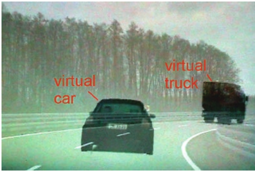
■ Fig. 10.19 View of the test subject through the HMD on the real track with simulated virtual vehicles. (From Bock 2008)
