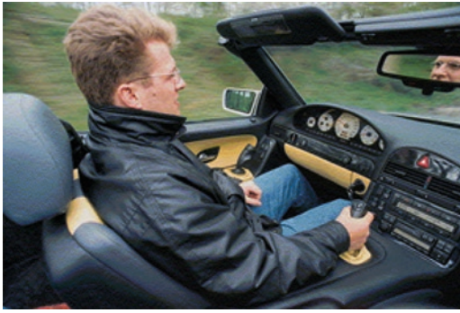
■ Fig. 6.63 Example for test vehicle with sidestick control (Mercedes 500 SL; Eckstein 2001)
