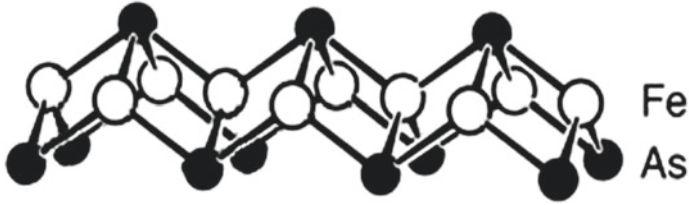
Fig. 10.1 Layers of FeAs (or similarly of FeSe) sandwiched between layers of lanthanum oxide and possibly doped with fluorine
