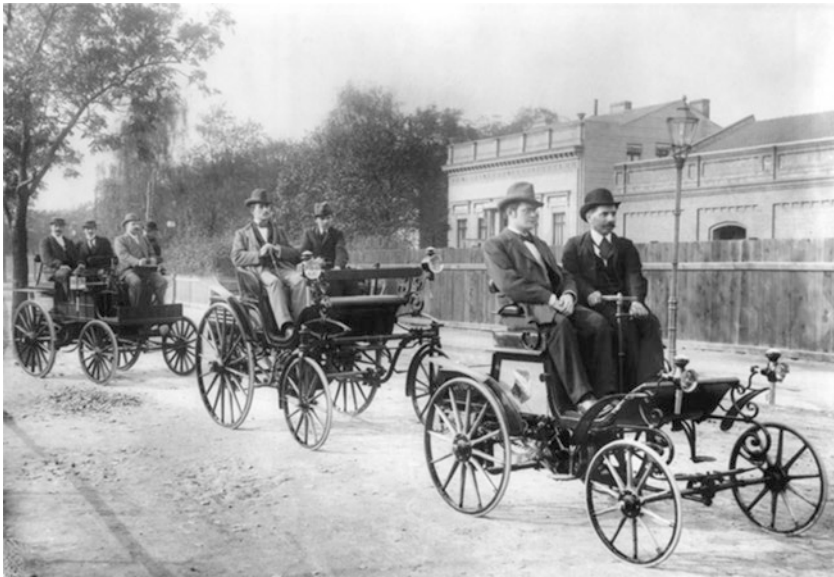
Fig. 2.1 The cars are still carriages, but equipped with motors. The manufacturer Lutzmann from Dessau presents various models in a motorcade, 1897. (Source: Landesbildstelle Berlin)
