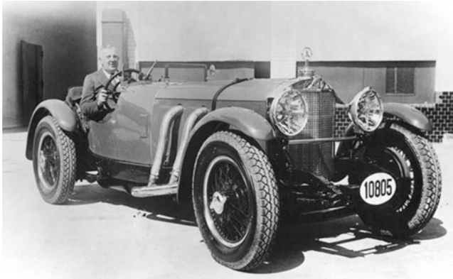
Fig. 2.5 In the Mercedes S sports car, the elongated engine block and the massive radiator demonstrated the power of the machine. A company specializing in automobile bodies equipped this one with designer elements such as the chrome exhaust pipes, which increased the prestige and made the car a medium of social distinction for the upper classes (1920s). (Source: Landesbildstelle Berlin)
