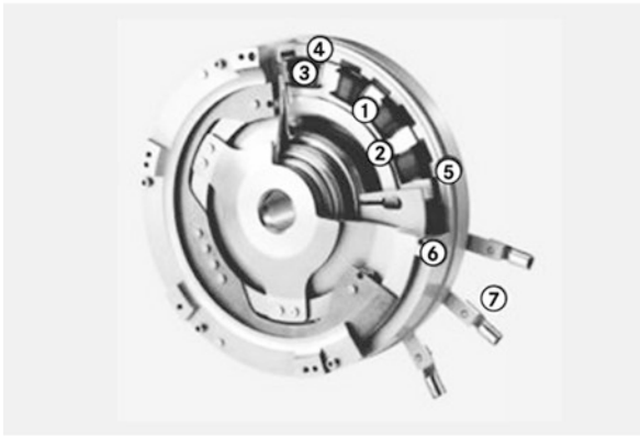
Fig. 6.3 Compilation of motor types. (a) Asynchronous motor (Source: Wallentowitz et al. 2010). (b) Synchronous motor with permanent magnets. (1) stator. (2) stator backs. (3) copper windings. (4) surface magnets. (5) Rotor core. (6) Rotor shaft in external rotor design. (7) High-voltage plug connection (Source: ZF-Sachs). Anschlussleitungen: Connection Cables; Luftfilter: Air Filter; Rad für Geschwindigkeitssensor: Gearwheel for Speed Sensor; Motorgehäuse: Motor housing; Rotor mit Kurzschluss­spule: Rotor with short circuit ring; Ständereisenpaket: Stator core; Lüfterrad: Cooling Fan Wheel; Ständerspulen: Three-Phase Windings
