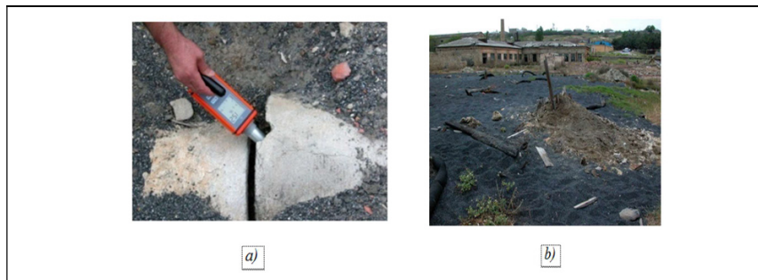
Figure 1: The measurements on the territory of Ramani plant (a) and object with coordinates N40°26'43,0"; E49°57'51,7", where EDR = 1450 \mu R/h (b)
