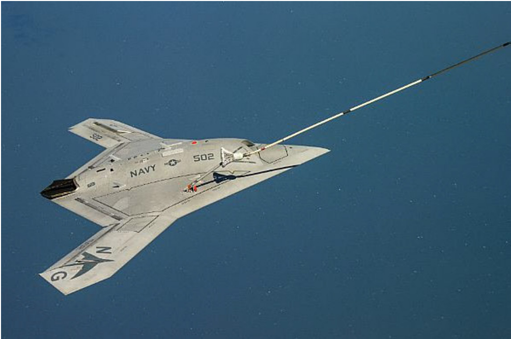
Figure 11-1: X-47B being refuelled while in-air, April 22, 2015
