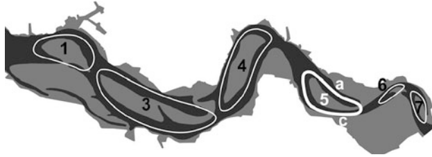
Fig. 6.11 The Schelde is intersected by sand plates and consists of multichannel system. Sediment is eroding and mainly relocated in so-called morphological cells. In the Schelde seven morphological cells have been identified. Within these cells the approach of morphological management will be applied by relocating the dredged material within these cells and not extracting from the system. Source: Deltares (2012)
