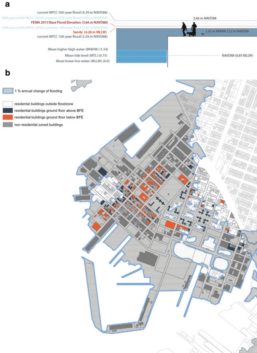
Fig. 9.4 Water levels at the Red Hook waterfront at the current 100-year flood level and projected flood levels at the 10-percentile and 90-percentile NPCC 2050 scenario. The dotted red line indicates the maximum level reached during hurricane Sandy ( upper picture ) and residential buildings in the 100 year flood zone with the ground floor below the base flood level (BFE) ( lower picture )
