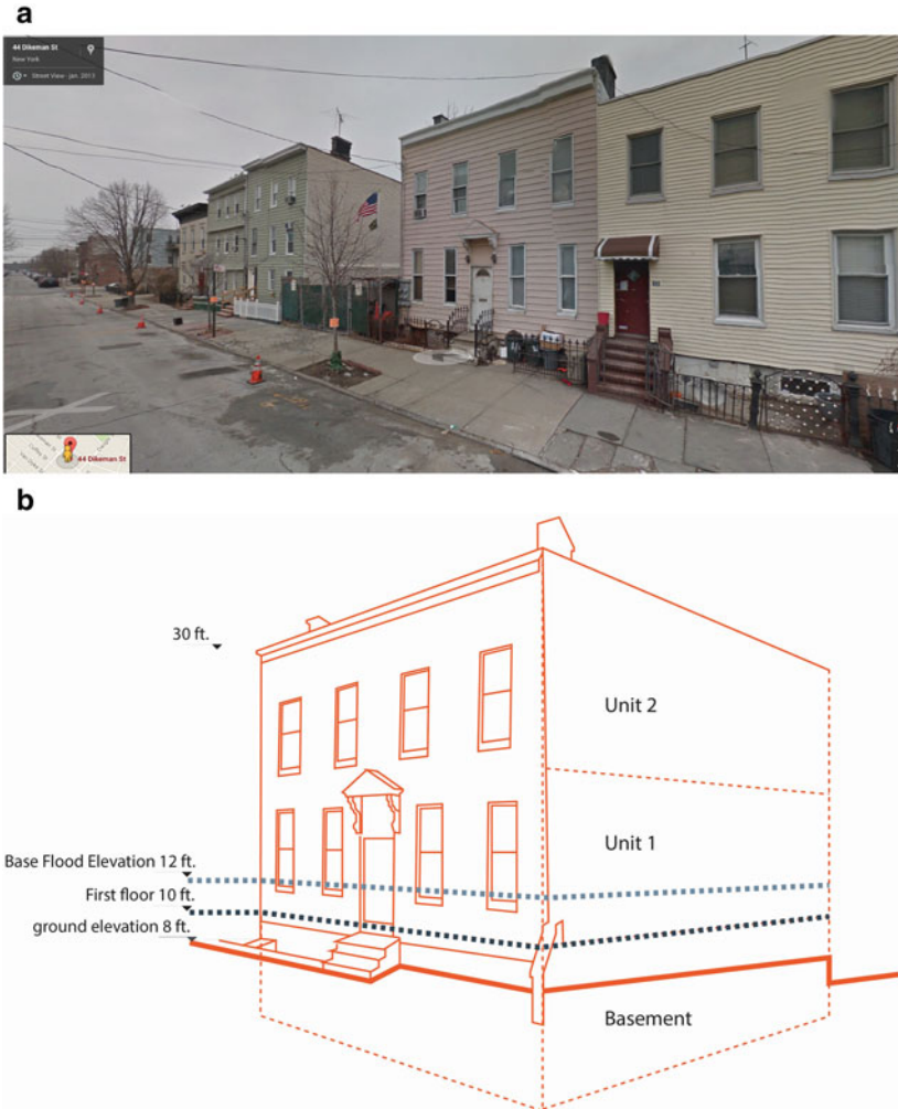
Fig. 9.5 Typical Red Hook building with semi below grade basement and ground floor apartment located below the base flood elevation (BFE) (Sources: upper picture Google street view, lower picture by author)
