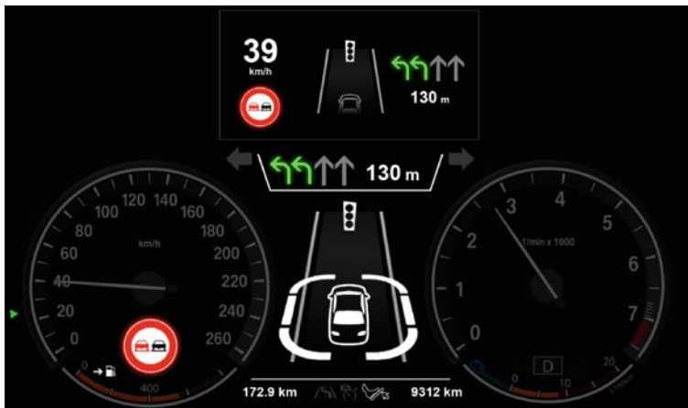
Fig. 7.19 The final concept with the head-up design ( top ) and the instrument cluster design ( bottom )
