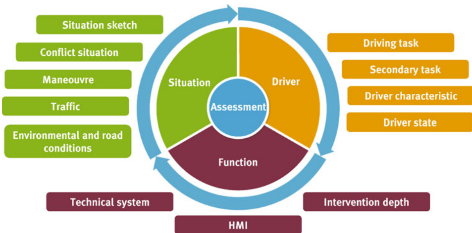
Fig. 2.1 Dimensions of the classification scheme for urban assistance scenarios. (Adopted from [2]; reproduced with permission from C. Purucker and A. Neukum)
