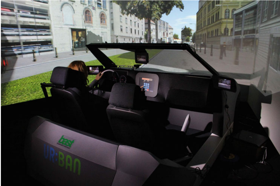
Fig. 25.2 The BASt static driving simulator used in the study
