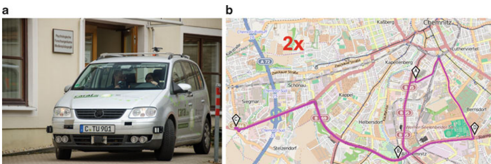
Fig. 11.1 Instrumented test vehicle VW Touran 2.0 TDI (a) and experiment route, 2×20 km in the urban area of Chemnitz, Germany (b). (OpenStreetMap contributors, 2016)
