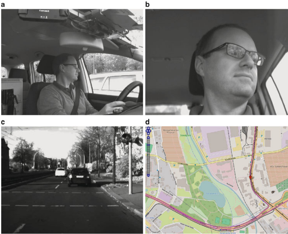
Fig. 11.2 Video examples front camera (c), interior camera (a), driver camera (b) and synchronised GPS-track (d). (OpenStreetMap contributors, 2016)
