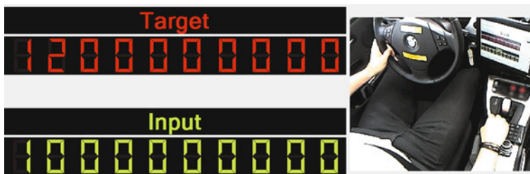
Fig. 10.4 Illustration of the used secondary task. Left picture shows the task representation on the display where the participant is requested to type the first digit "1" and second digit "2". The remaining digits are not shown yet, instead their fields are initialized with "0". Right picture shows a participant conducting the secondary task while driving
