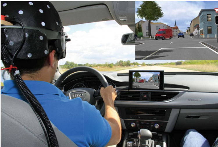
Fig. 25.4 The UniBw Vehicle-in-the-Loop (VIL) used in the study
