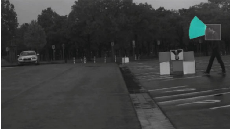
Fig. 14.11 Pedestrian Head Orientation Estimation to detect the pedestrian’s intention to cross for earlier warning system
