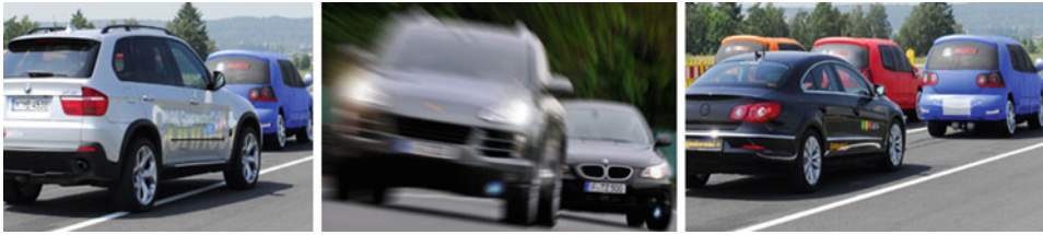
Fig. 1.7 Automatic emergency braking taking evasive action by the driver into account. (From AKTIV-AS AGB)
