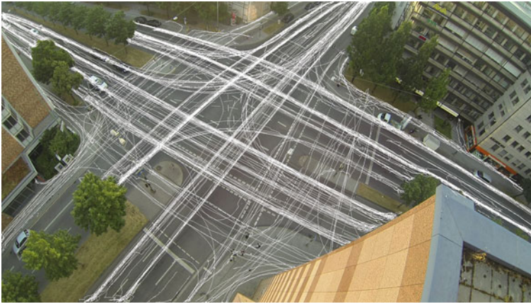
Fig. 18.2 Trajectory data extracted from a five minute video segment using Traffic Intelligence [18]
