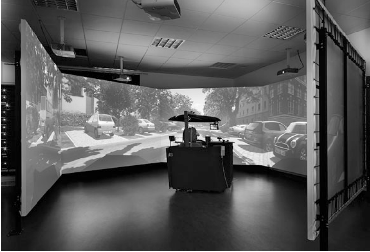
Fig. 22.2 Static car driving simulator
