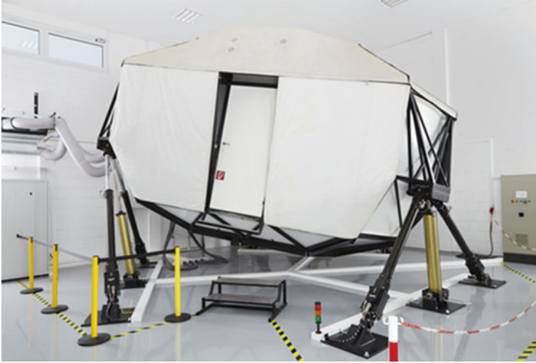
Fig. 25.3 The WIVW dynamic driving simulator used in the study
