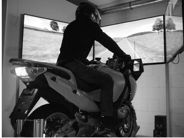
Fig. 22.1 Static motorcycle riding simulator
