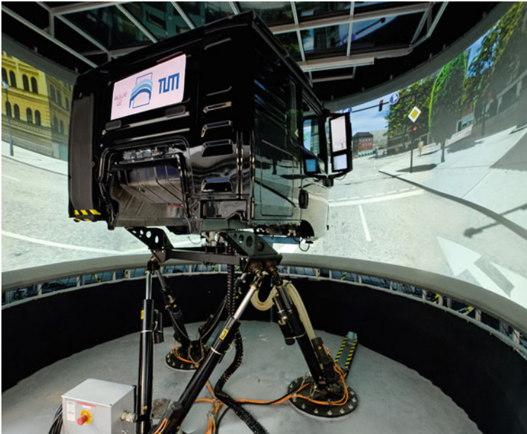
Fig. 6.5 Dynamic truck driving simulator at the Institute of Automotive Technology, TU Munich, Germany
