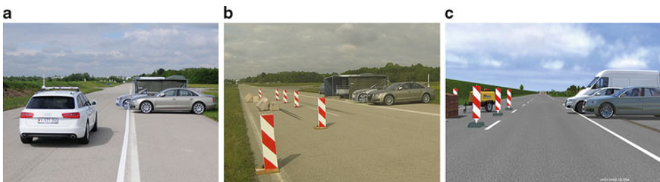
Fig. 26.2 Driving Situation on the test track (a), with occupied opposite lane (b) and in the VIL (c)
