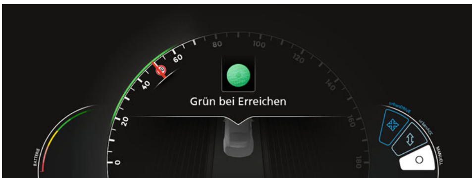
Fig. 20.1 HMI draft of the currently developed urbanDRIVE at DLR. Drivers are advised to travel at a certain speed in order to cross the intersection on a green light [16]
