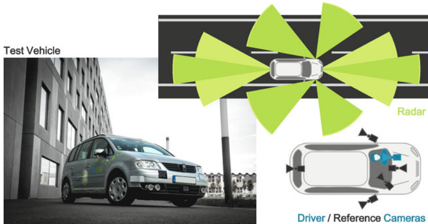
Fig. 12.9 Test vehicle and sensor configuration
