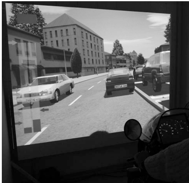
Fig. 23.1 Confederate in the connected motorcycle-car multi-driver simulation. The projection includes augmented reality elements displaying the distance to the vehicle ahead in meters and seconds as well as recommended thresholds indicated by arrows
