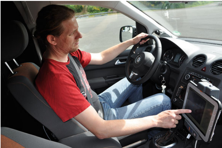
Fig. 29.1 Experimental setup of the driver's cabin including an additional touch screen for executing secondary tasks
