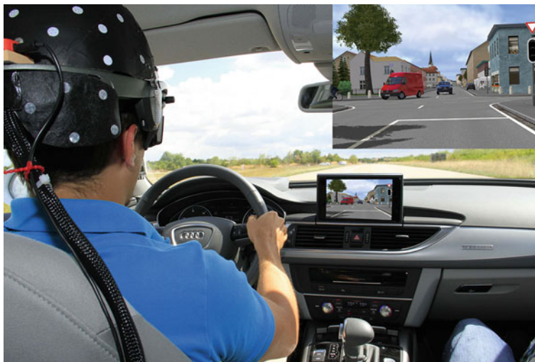
Fig. 26.1 Vehicle in the Loop (VIL). The picture on the top right shows the driver's view
