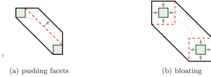
Fig. 12. An approximation \Omega_0 that covers \mathcal{X}_t for t \in [0, \delta] can be obtained from the convex hull of \mathcal{X}_0 and \mathcal{X}_\delta and compensating for the curvature of trajectories
