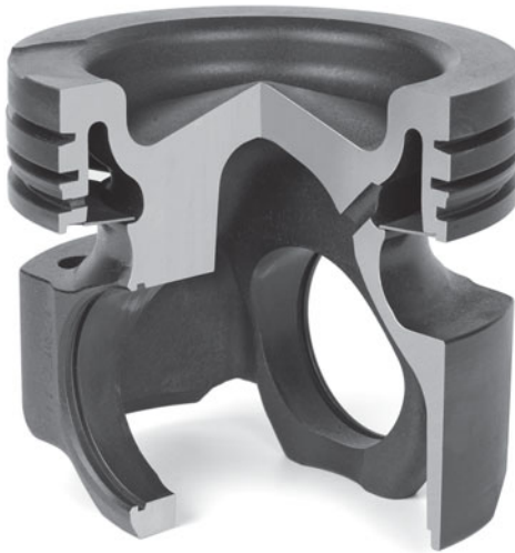
Figure 5.12: MONOTHERM® piston with cover plate to close the cooling gallery
