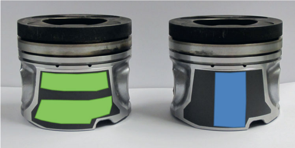
Figure 7.53: Horizontal orientation (left, green) and vertical orientation (right, blue) of the reduced bearing skirt areas (height of the supporting profile 100–200 \mu\text{m} )
