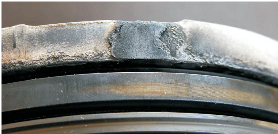
Figure 7.71: Carbon buildup on the top land of a commercial vehicle piston
