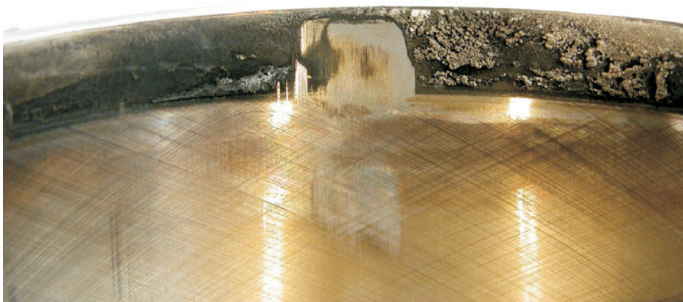
Figure 7.72: Cylinder area polished by the buildup of carbon on the top land
