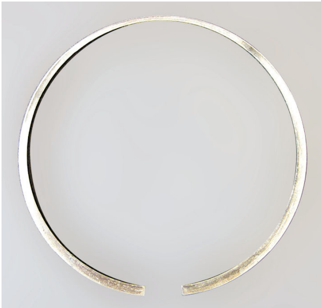
Figure 7.68: Example of extreme single-sided wear of 1st piston ring
