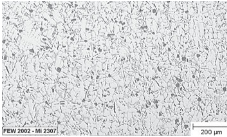
a) Eutectic AlSi alloy M142 (representative for M124 and M174+ as well), casting state with granular structure
