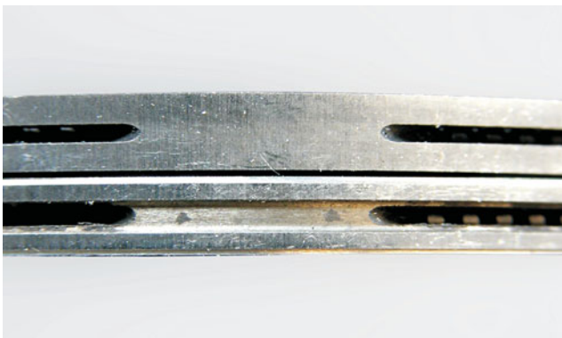
Figure 7.69: Example of extreme wear of two oil control rings
