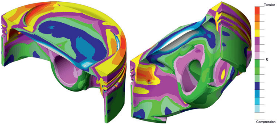
Figure 3.7: Thermally induced stresses in a piston for a passenger car gasoline engine with port fuel injection
