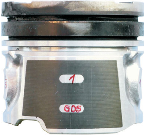
Figure 7.60: Piston with GRAFAL® coating, with recesses for measuring the skirt profile
