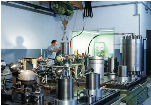
Figure 6.4: Hydropulsator tests on piston
