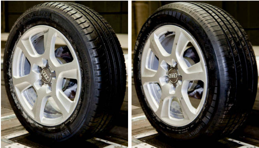
Figure 8: Standard production tyre (left) and tyre with optimized aerodynamic characteristics (right) [7]
