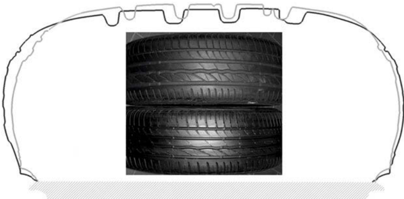
Figure 9: Tyre shape for two tyres of the same type (205/55 R16) [7]
