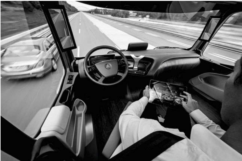
Fig. 6: The driver works with the tablet PC and the driver's seat is swiveled through 45°
