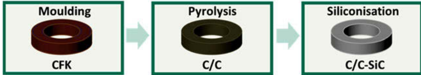
Figure 1: Production of ceramic C/C-SiC composite materials by means of LSI
