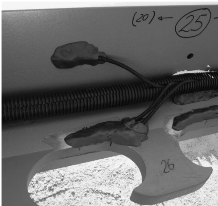
Figure 18: Protected strain gauges, covered with 2-component adhesive (PS-adhesive) and permanent elastic cement (AK22)
