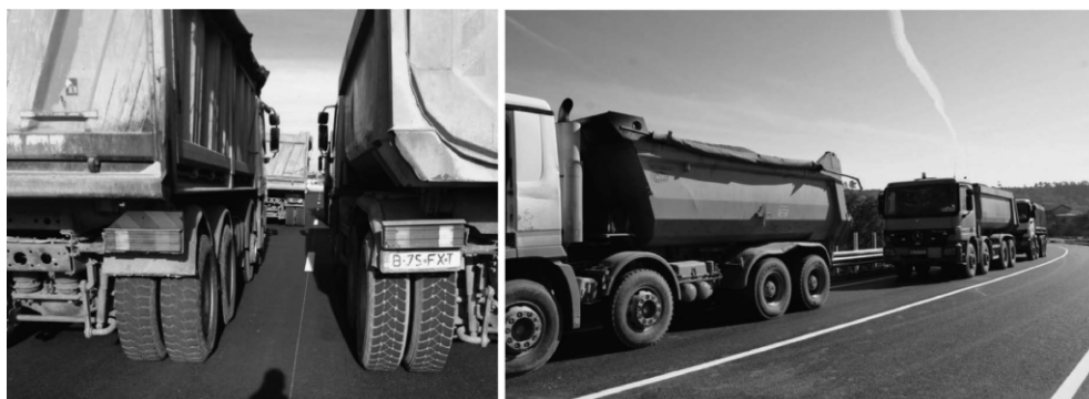
Figure 29: Preparatory actions for the load test convoy – LC2
