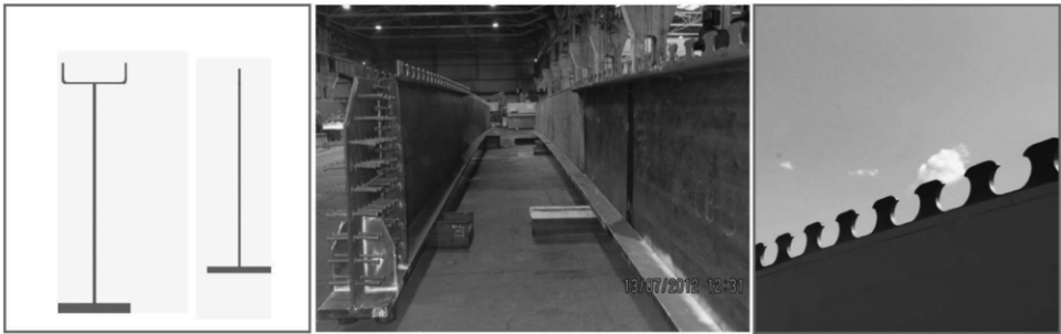
Figure 9: The steel girder type sections; Steel girders in the workshop; the cutting line geometry of the composite dowels.
