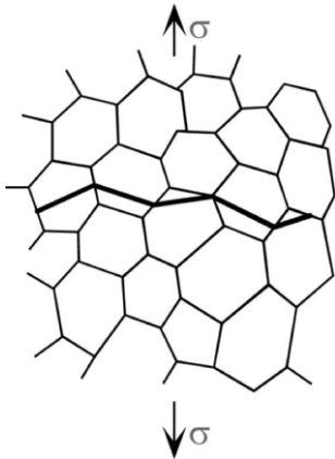
Figure 12: Model of crack propagation in the crystal lattice
