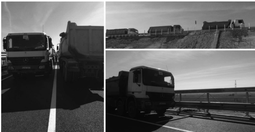
Figure 13: MAN TGA convoy – front view, lateral view; dynamic load test MAN TGA vehicle.
