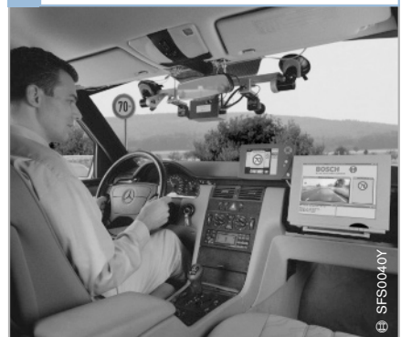
3 Experimental vehicle featuring "road sign recognition using video sensors"
