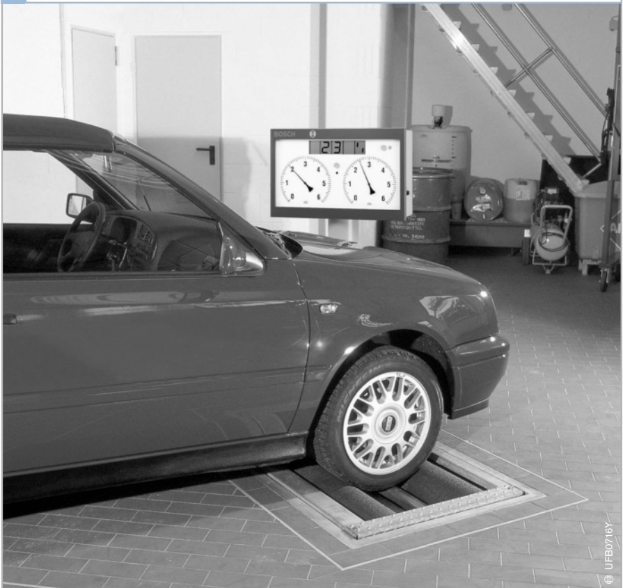
1 Testing brakes on a brake tester
