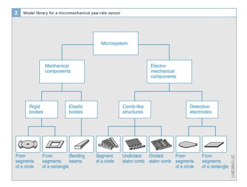
Basic issues can often be clarified by producing relatively simple models of the components. If more detail is required, more refined component models are needed. The detailed models focus mainly on a specific physical domain:
