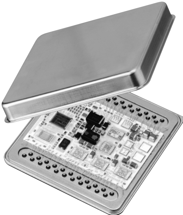
9 Microhybrid ECU in steel housing
