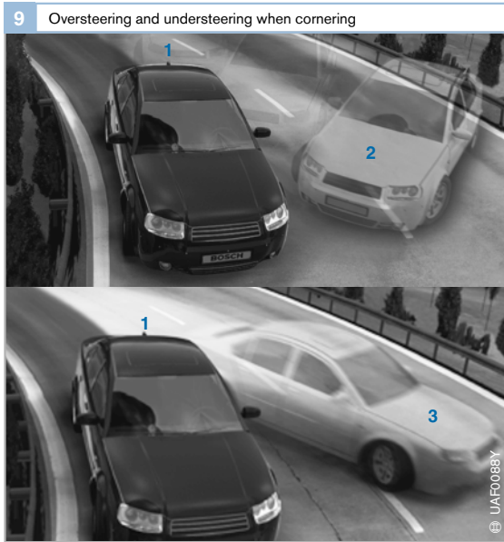
Fig. 9 1 Vehicle with ESP 2 Oversteered vehicle without ESP 3 Understeered vehicle without ESP
