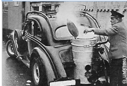
22 Wood-gas generator system on a 1936 Adler Diplomat
