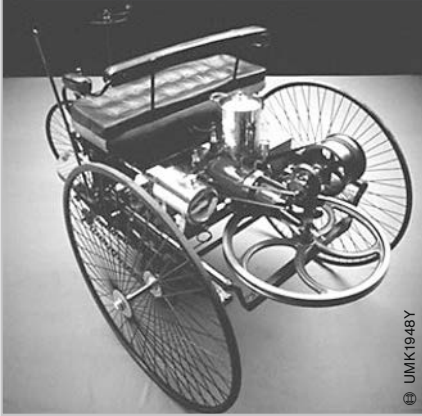
5 Benz Motor Carriage with surface carburetor (vertically positioned)
