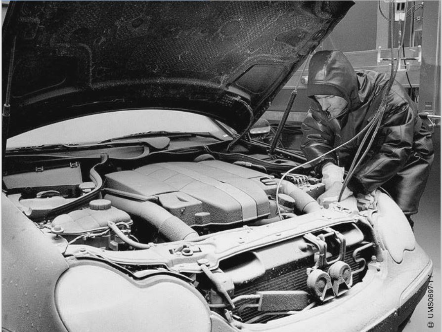
4 Recording cold-starting response in the cold room
