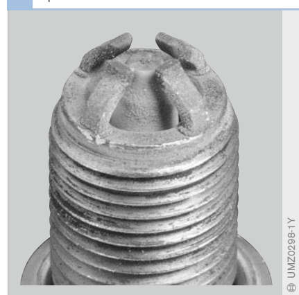
9 A Platinum+4 spark plug after 800 hours of operation
