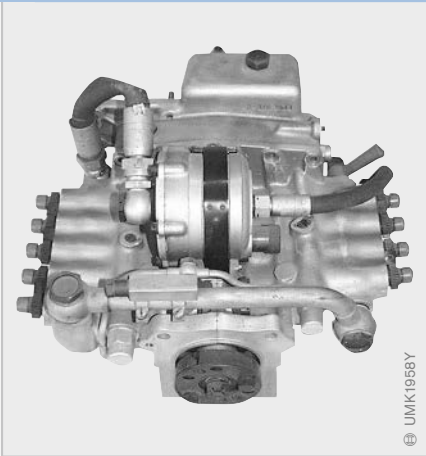
15 Bosch fuel-injection pump in "boxer" (reciprocal) variant (length approx. 35 cm)
