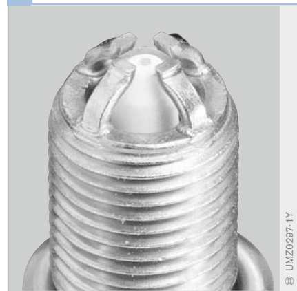
8 Profile of a new Platinum+4 spark plug
