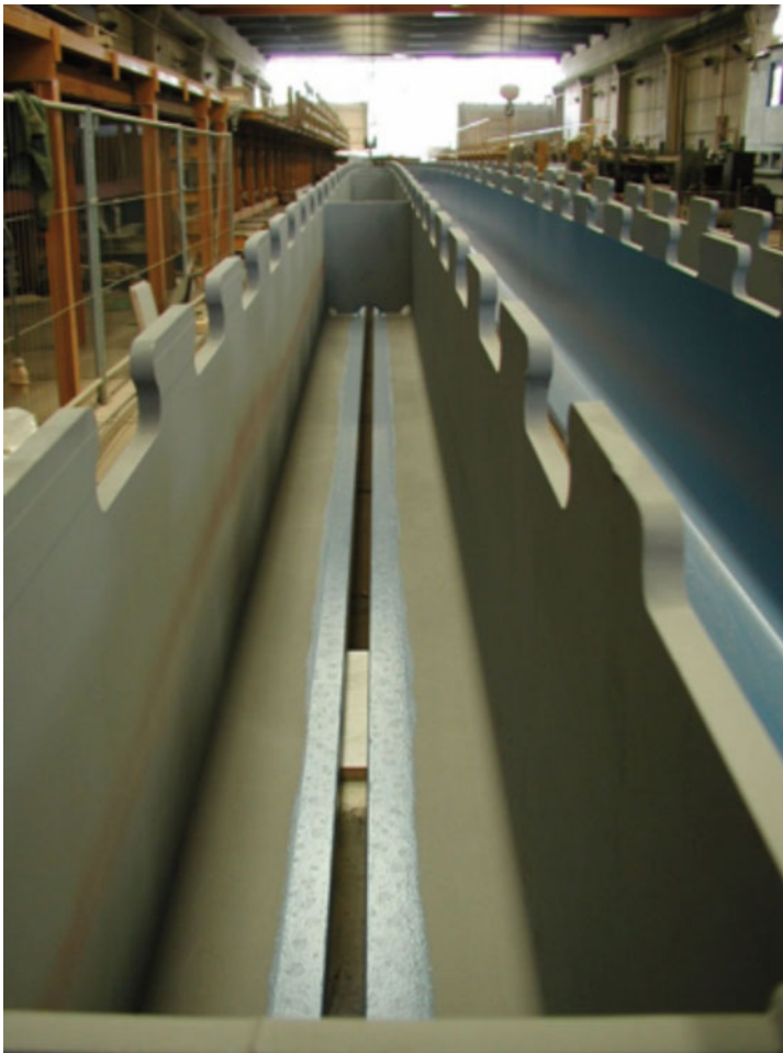
Figure 3: Cut (halved) rolled sections with PZ-geometry of the dowels and coating in the prefabrication plant
