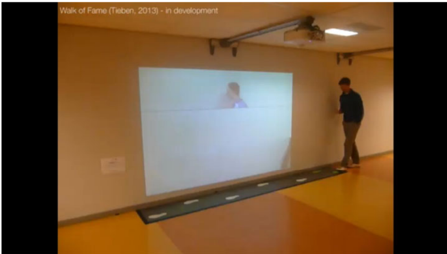
Fig. 4: The Walk of Fame. Walking on the carpet starts a recording. Partial playback results in funny combinations of heads, trunks and legs moving down the hall. The installation elicits repetitive walking to perfect the coordination of displayed body-parts.
