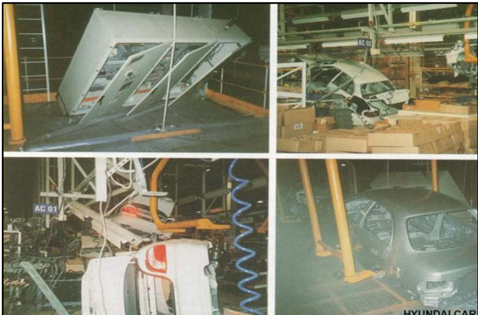
Figure 2: Equipment damage at Hyundai-Assan car factory (after Milli-Re)
