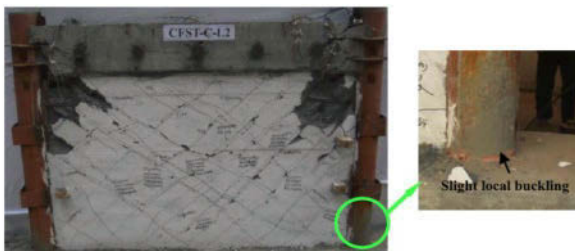
Figure 5: Failure mode of Hybrid wall. (Adopted from Liao et al. 2009 [16])
