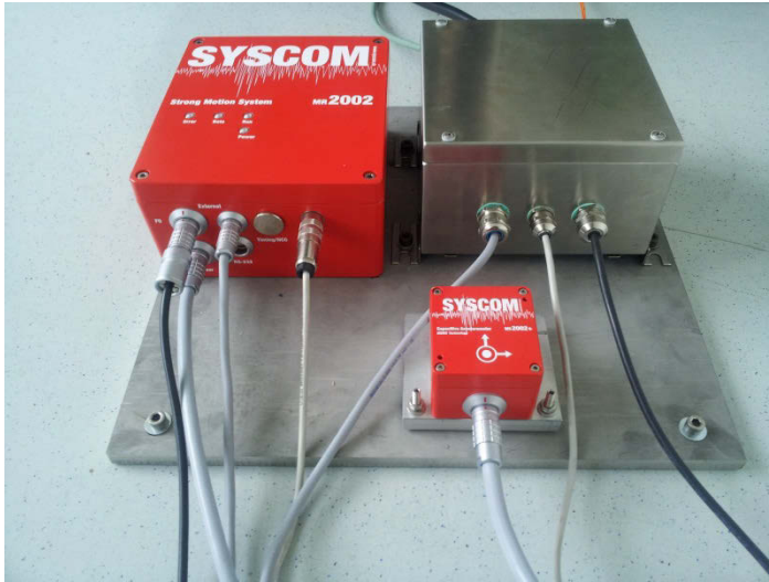
Figure 3: Strong motion recorder (MR2002), Accelerometer (MS2002) and stainless steel junction box mounted on a platform
