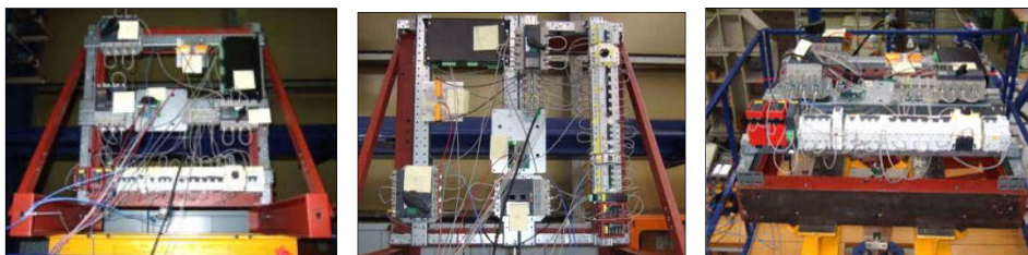
Figure 6: Orientation of specimen during tests for excitation of: vertical (left), horizontal-x (middle) and horizontal-y (right) direction
