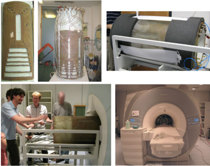
Figure 3.17: Construction of the PatLoc human head insert coil. From left to right, top row: The new coil consisted of several identical wire elements, which differentiated significantly from the elements of the PatLoc prototype coil. These elements were mounted on a cylindrical former, water cooling was added and the components were fixed with epoxy resin. Bottom row: With the RF coils inside, the coil was then introduced into the scanner bore.
